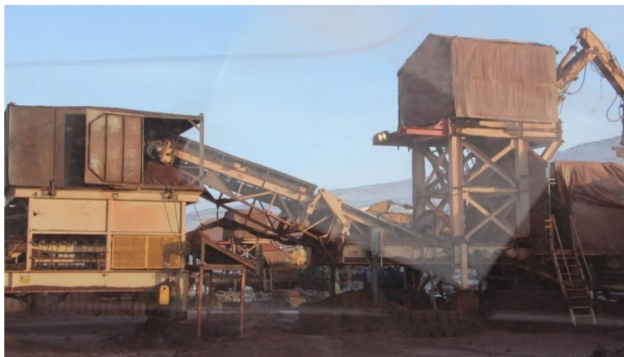
Photo 8: Shroud installation at crusher facility
