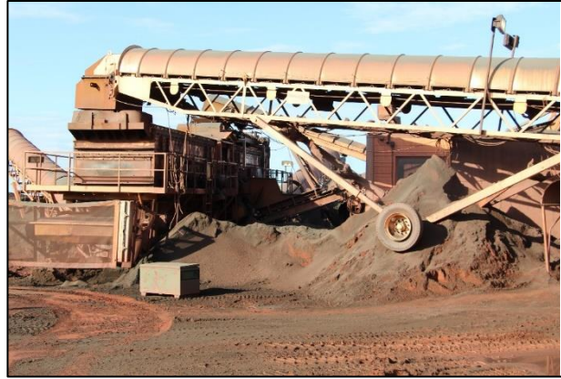
Photo 15: Fine Ore Build-Up Beneath the Crusher Conveyor Belts
