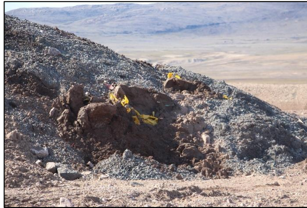
Photo 34: Few Remaining Synthetic Liners in the Landfarm
