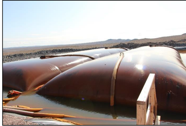
Photo 7: Geotube Bladders used for Particle Separation of Waste Rock Effluent
