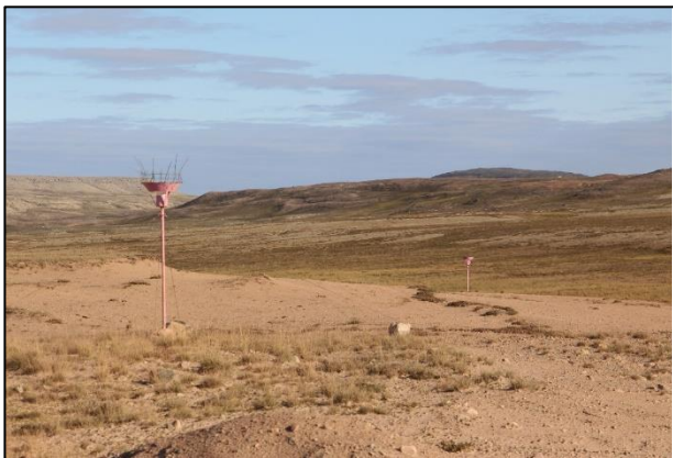
Photo 44: Dust Fall Stations at various distances leading away from the Tote Road
