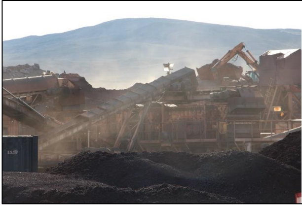
Photo 14: Dust Emissions from the Crusher Facility at the Mine Site
