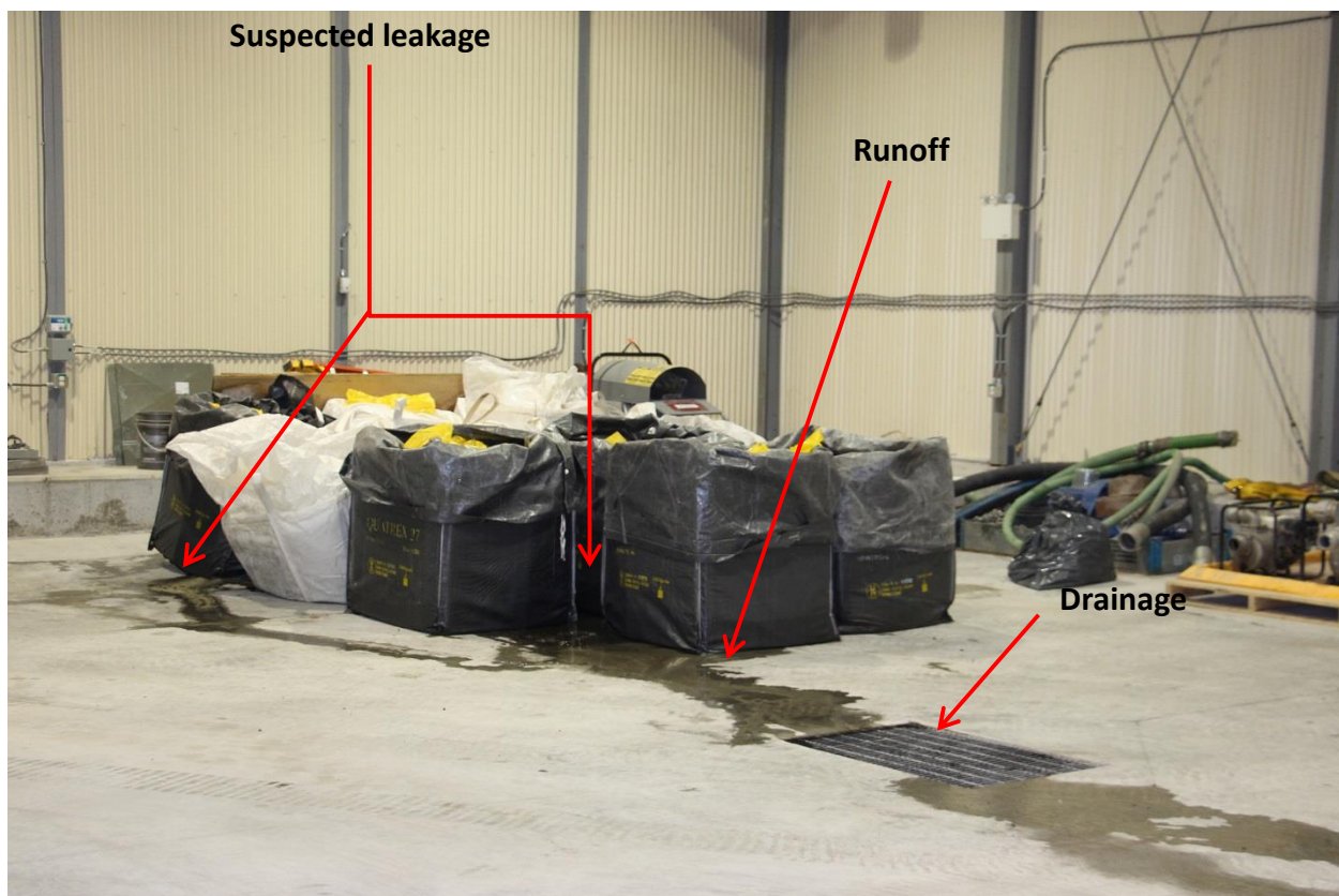
Picture 36. Runoff of oil contaminated discharge to waste drain
