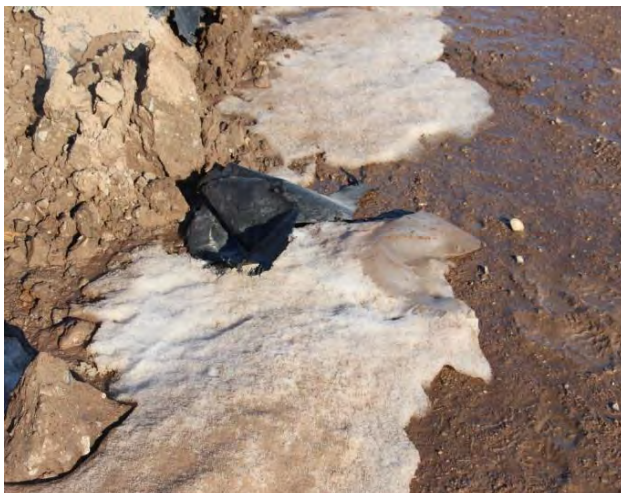
Picture 49: Pieces of liners blown away
