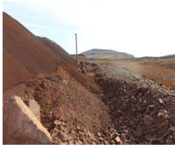
Picture 21: Ore pad expansion blocking drainage
