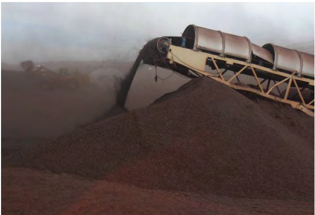
Photo 12: Missing cover from end of conveyor
