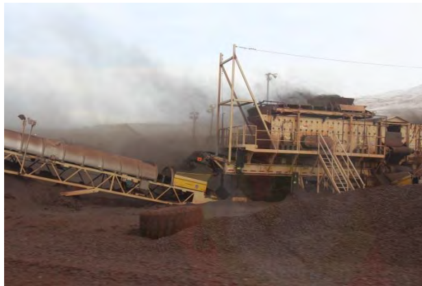
Photo 13: Dust from shaker and transfer points
