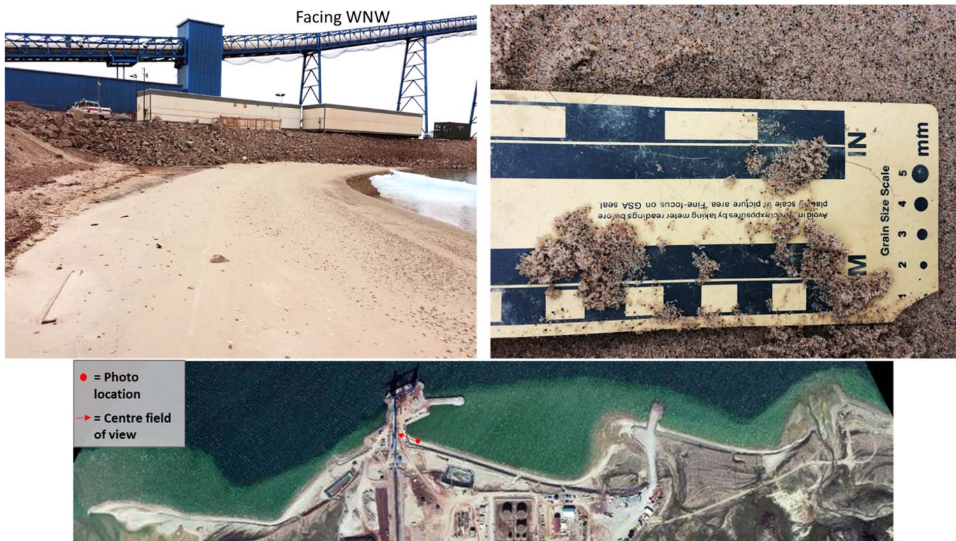
Figure A-2.9: Fine sand accretion along the eastern side of the ore dock riprap.
