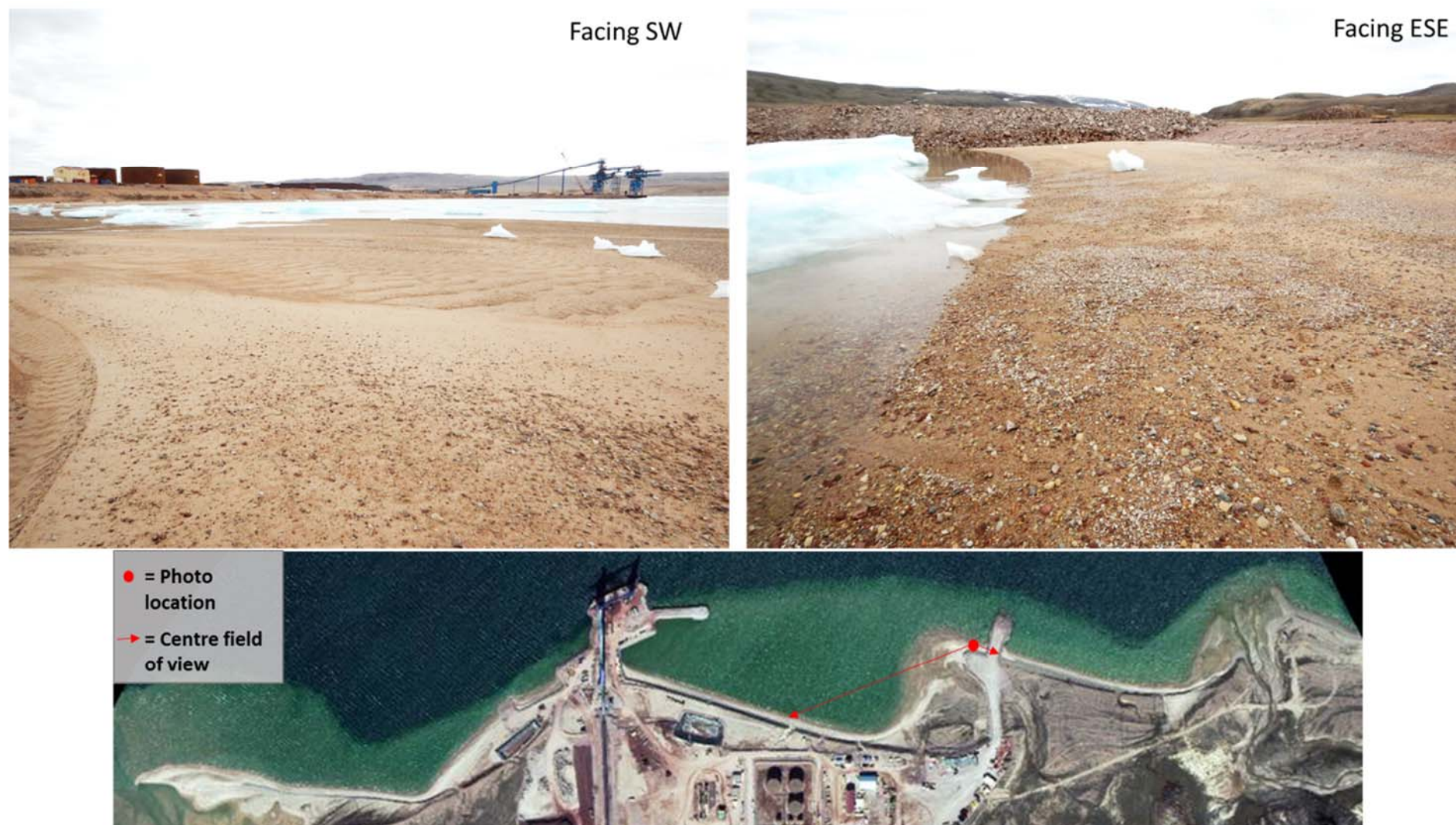
Figure A- 2.3: Western accretion of medium fine sand along perpendicular riprap and ridge and shore perpendicular bedforms along spit feature.
