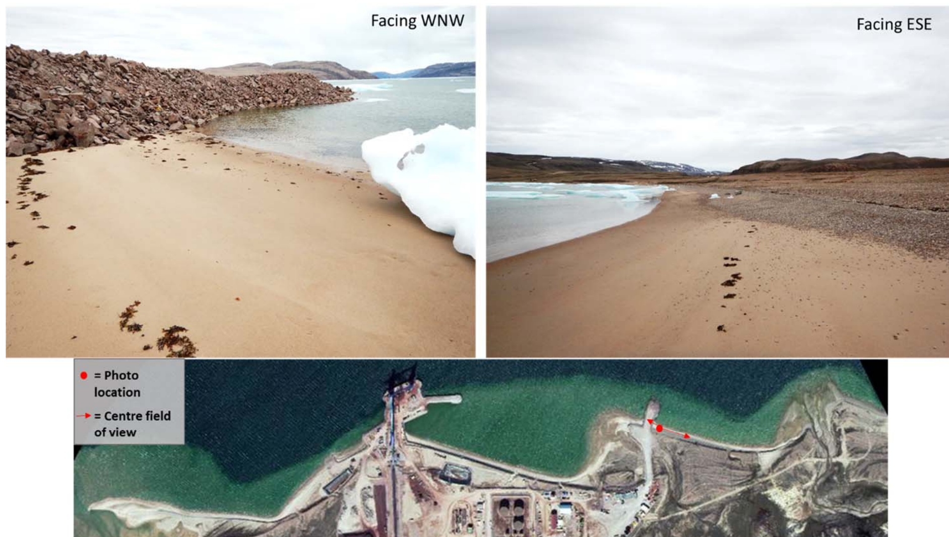
Figure A- 2.2: Eastern accretion of fine sand along perpendicular riprap.
