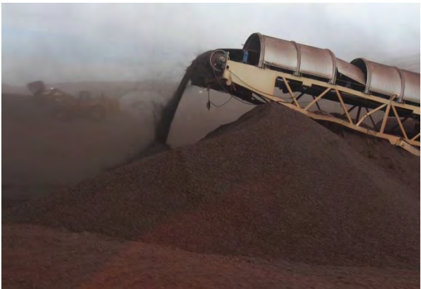
Photo 12: Missing cover from end of conveyor
