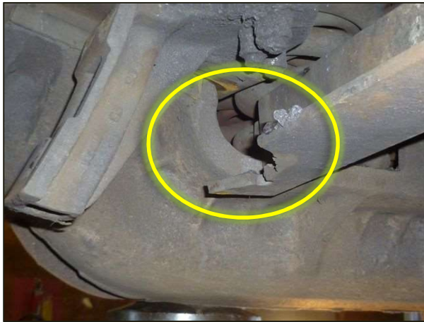
Figure Y: Worn brake beam
