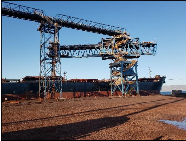
Barge loading area noting conveyor belts and chutes
