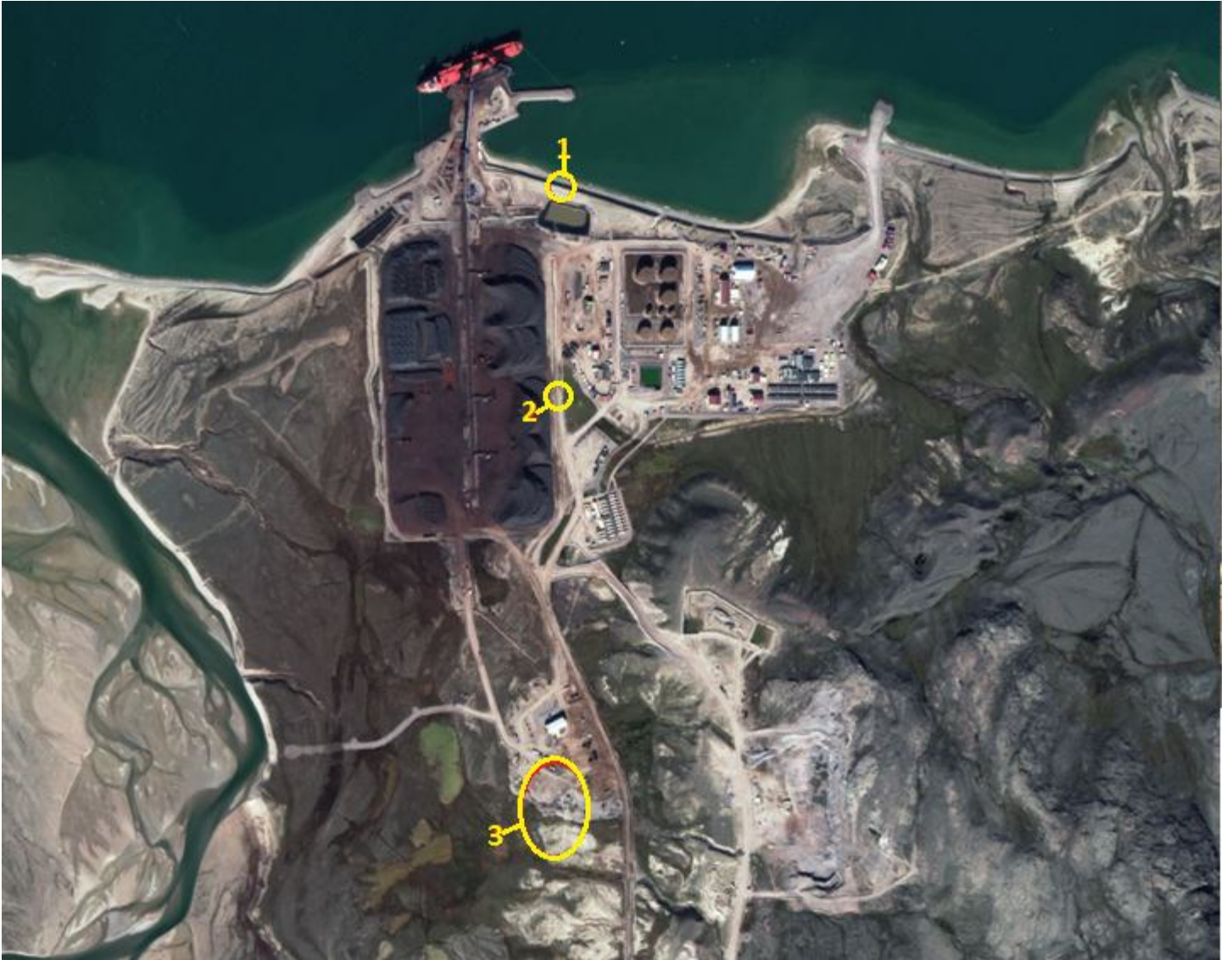
Figure 4: Item 1: Washout from East sedimentation pond. Item 2: location of water infiltrating ditches, the old snow dump and sampling location. Item 3: approximate location of the Camp lay-down Pad
