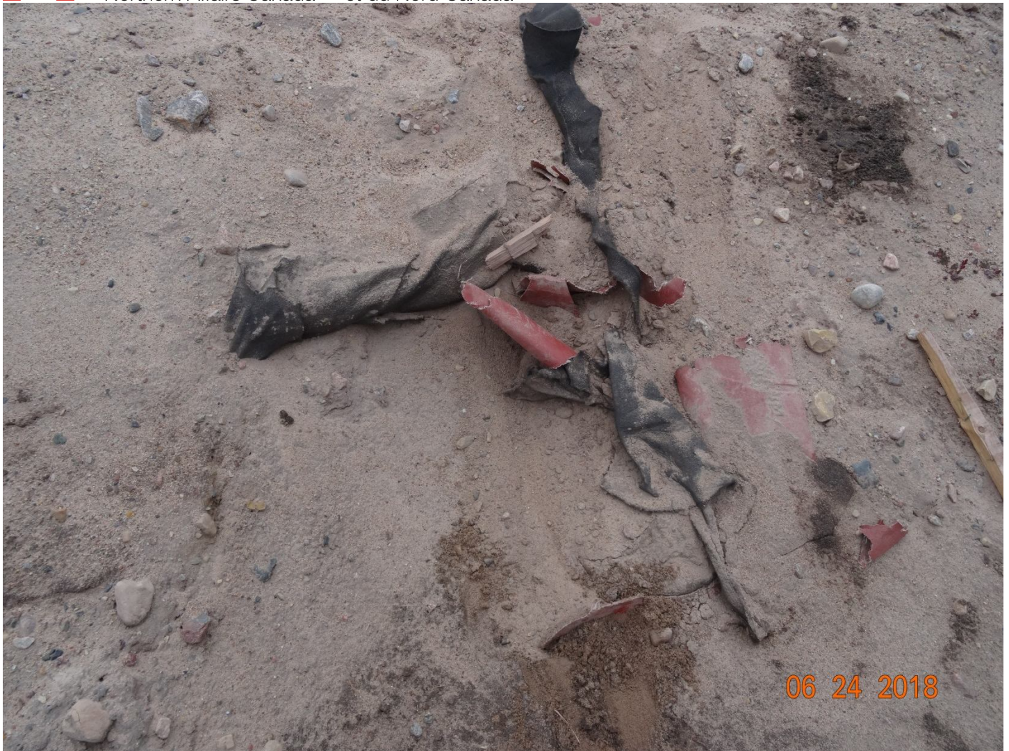
Figure 6: Hazardous waste secondary containment liner rip.
