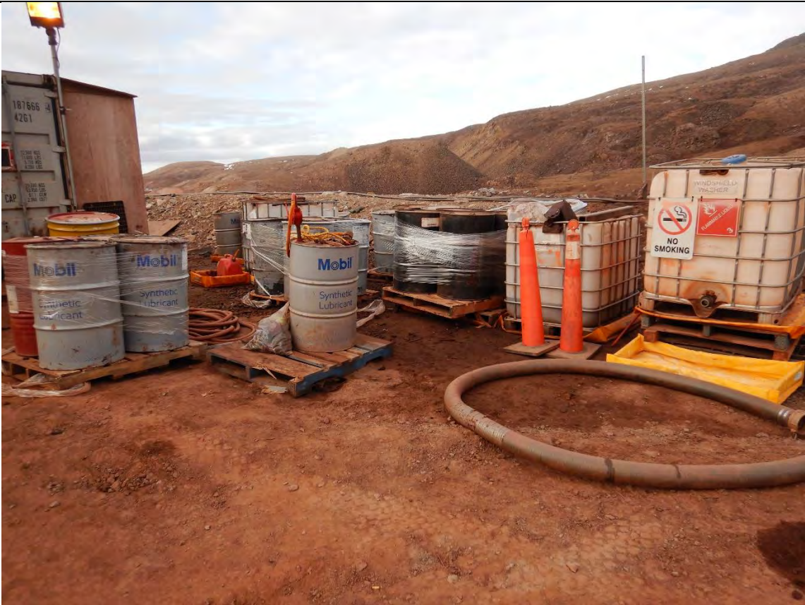
Description: hazardous material outside of containment, in damaged containment and staining in the area.
