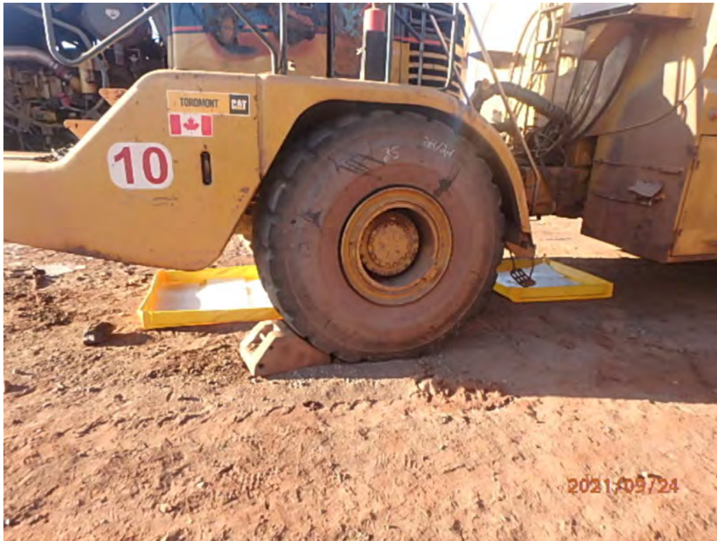
Photo 11 – Spill Trays beneath Heavy Equipment at the KM104 Laydown – September 2021
