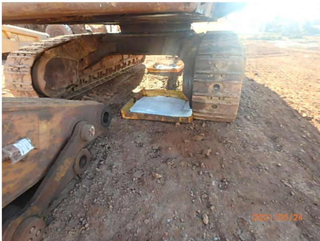
Photo 12 – Spill Trays beneath Heavy Equipment at the KM104 Laydown – September 2021
