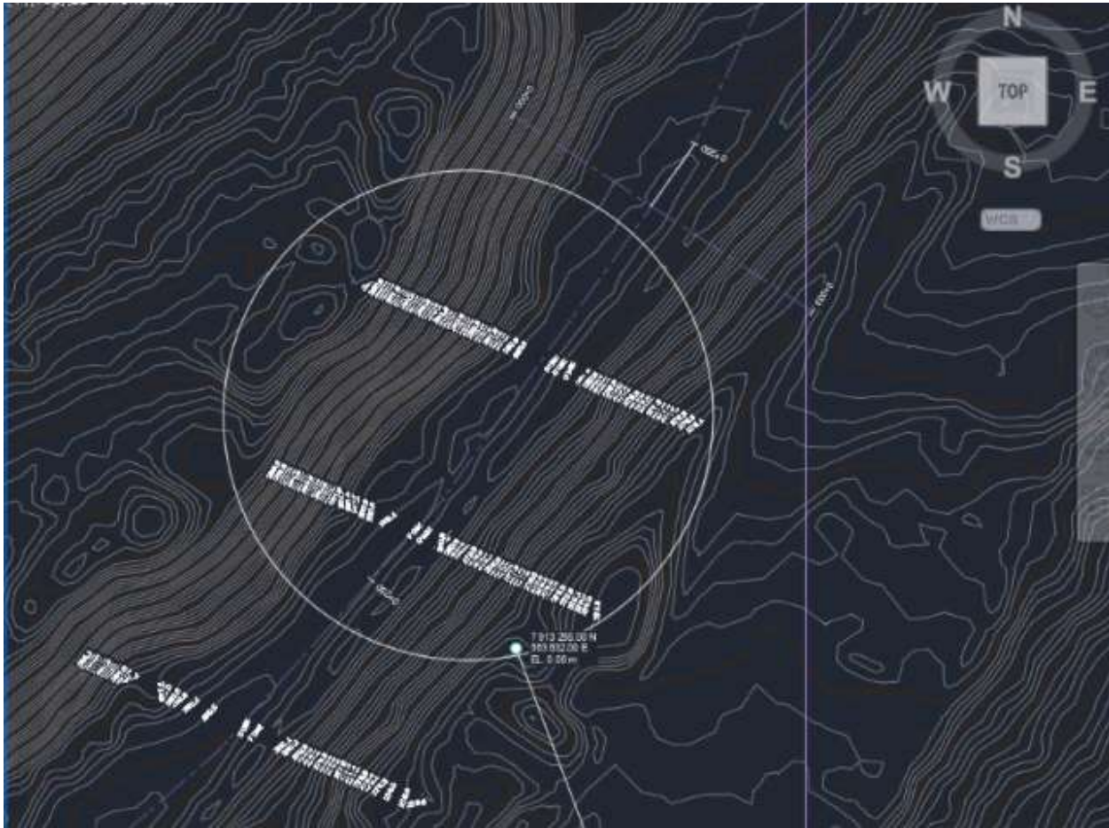
Figure 3 As-built Survey at MS-106OS-02 Showing a Low Spot
