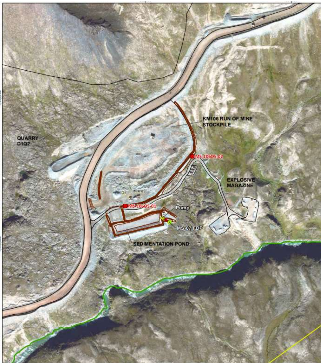
Figure 1 KM106 Stockpile and Pond Showing Seepage Locations (Baffinland, 2021)
