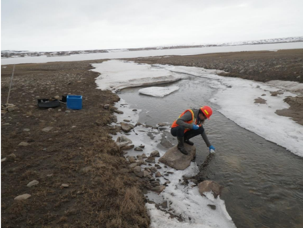
Photo 3 – May 30 th 2016. Daily sampling and monitoring of Camp Lake Tributary #1 discharge at Camp Lake outfall.
