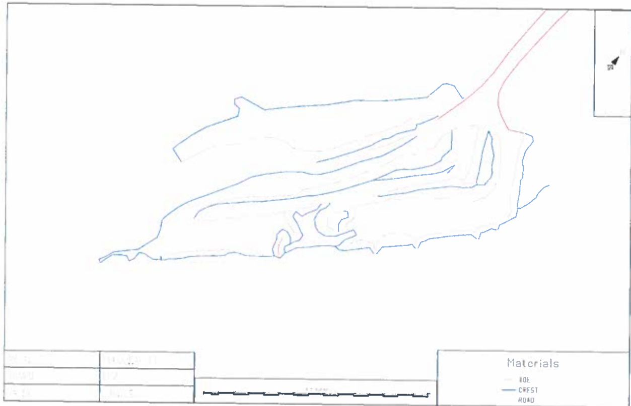
FIGURE 1 PLAN VIEW OF THE BULK SAMPLE PIT SHOWING THE TOE, CREST AND ACCESS ROAD.
