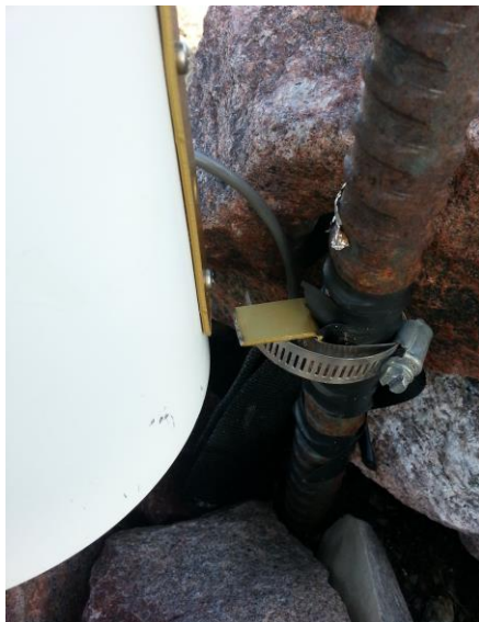
Figure 3: Milne TE525M with Broken mounting bracket
