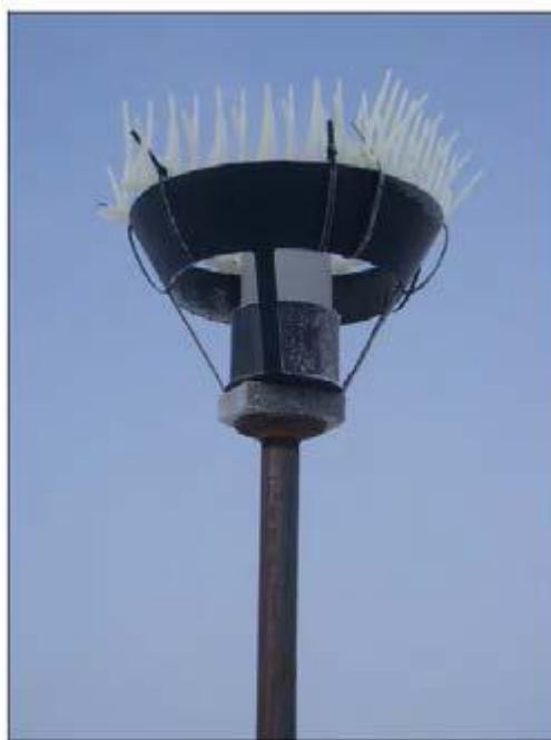
Photo 1: Dustfall collector sampling apparatus (from Rescan 2012).
