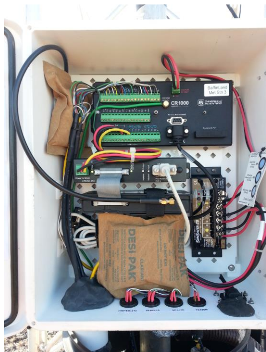
Figure 6: Inside Milne datalogger enclosure
