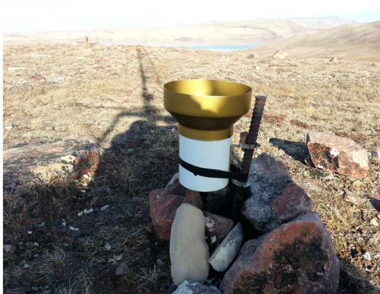
Figure 4: Milne TE525M showing repair of mounting bracket using electrical tape
