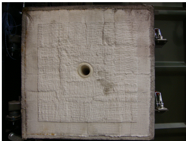
Secondary Door (refractory lined)
