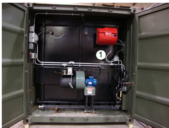
Primary Chamber Burner Flexible lines (1 Above)
