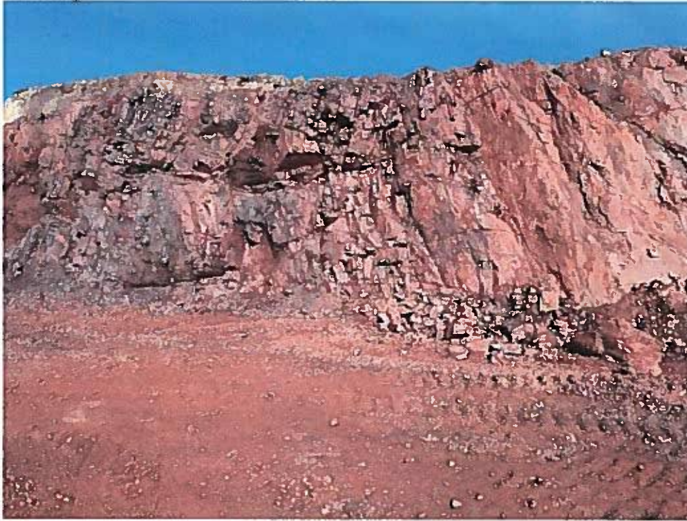
Photo 4: 10m high internal wall on outside edge of 640 Bench. Overburden across top of bench is raveling now that it has thawed.
