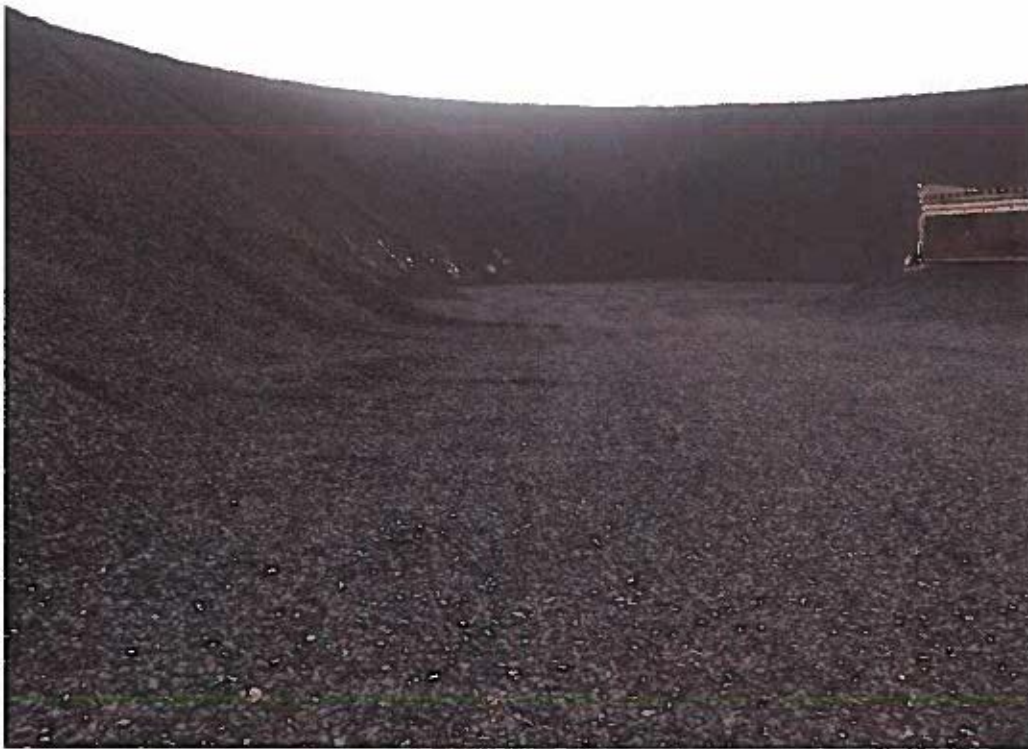
Photo 6: 18m high angle of repose stockpile with frost on surface
