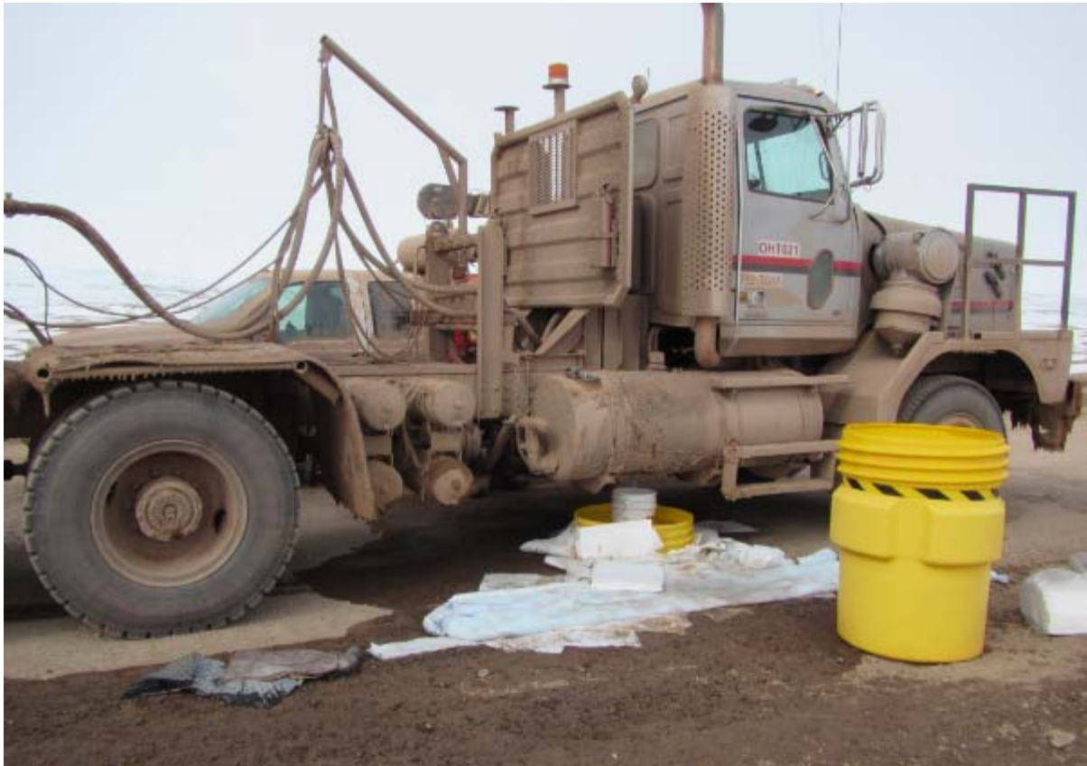
Photo 1 - Source of release – Ore Haul Truck Fuel Tank
