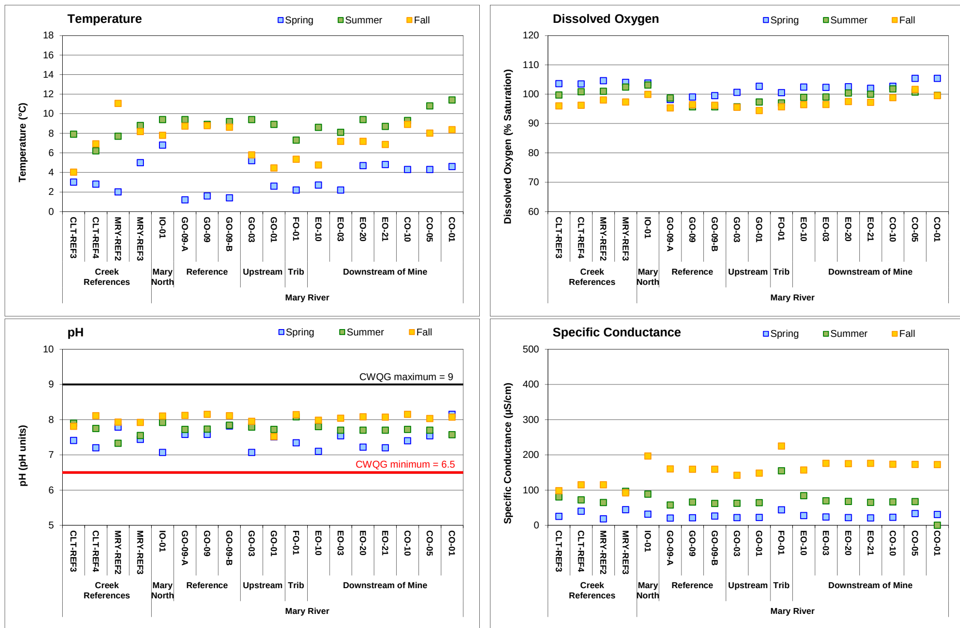
Figure C.19: Comparison of in-situ water quality variables measured at Mary River water quality monitoring stations in spring, summer, and fall 2016, Mary River Project CREMP.
