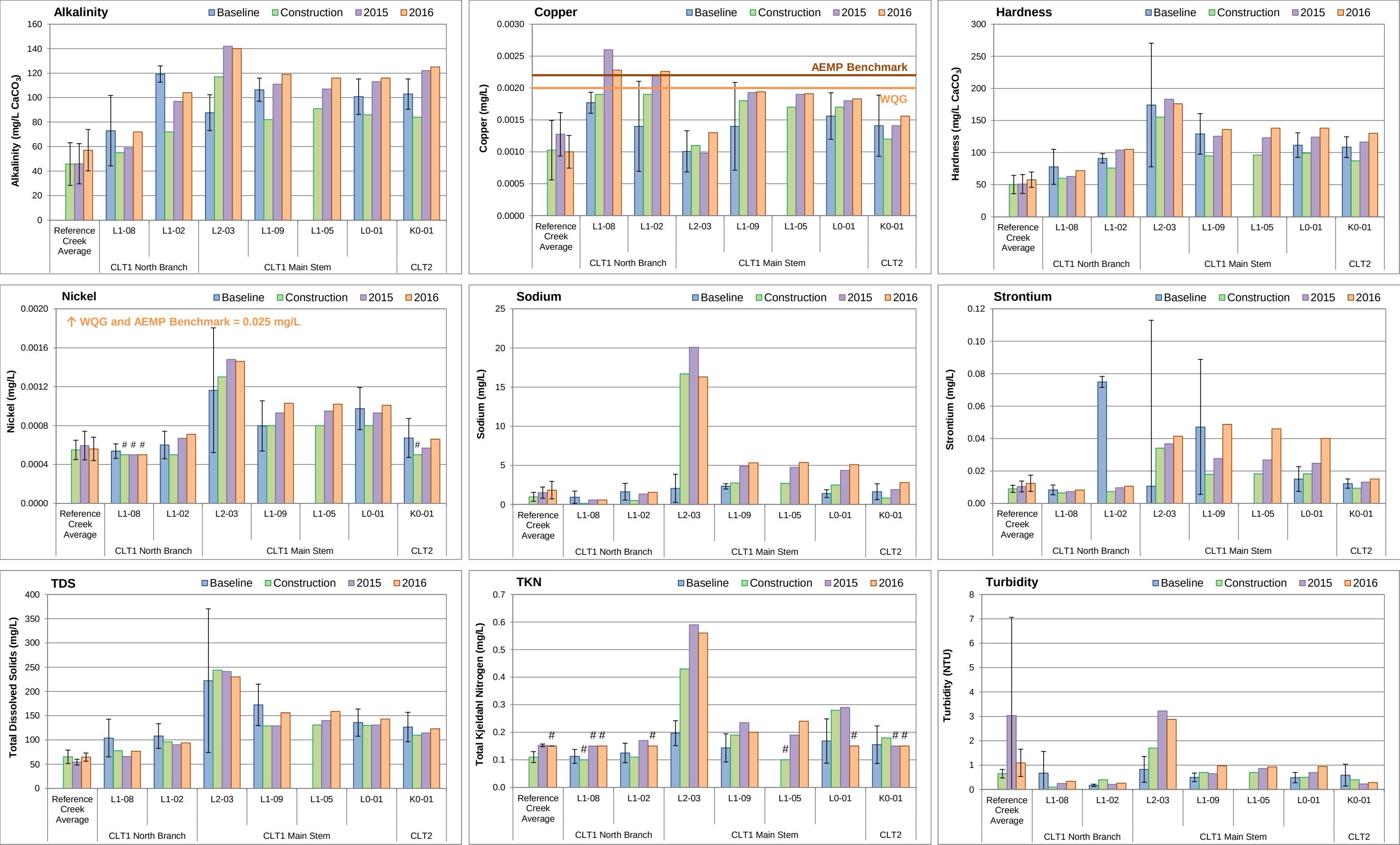
Figure C.2: Temporal comparison of water chemistry at Camp Lake Tributary 1 (CLT-1) and Tributary 2 (CLT-2) for mine baseline (2005 - 2013), construction (2014) and operational (2015, 2016) periods in the fall. Values represent mean \pm SD. Creek reference includes the CLT-REF and MRY-REF series stations (mean \pm SD; n = 4). Pound symbol (#) indicates parameter concentration is below the laboratory method detection limit. See Table 2.2 for information regarding Water Quality Guideline (WQG) criteria. AEMP Benchmarks are specific to the Camp Lake Tributaries.
