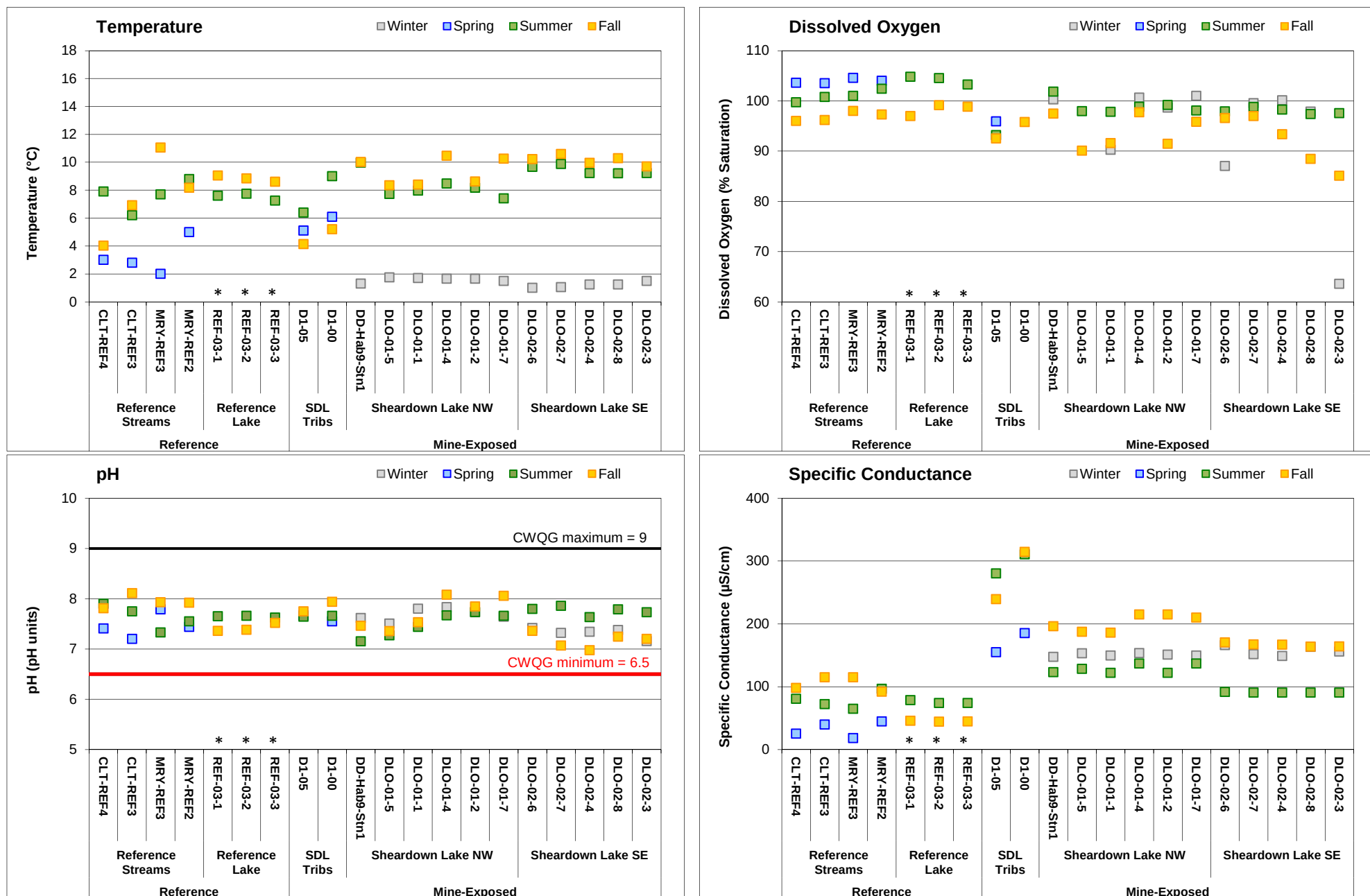
Figure C.8: Comparison of in-situ water quality variables measured at Sheardown Lake system water quality monitoring stations in winter, spring, summer, and fall 2016, Mary River Project CREMP. Lake values represent mean of surface and bottom in-situ water quality measurements. * Reference Lake 3 (REF-03) was not sampled in winter.
