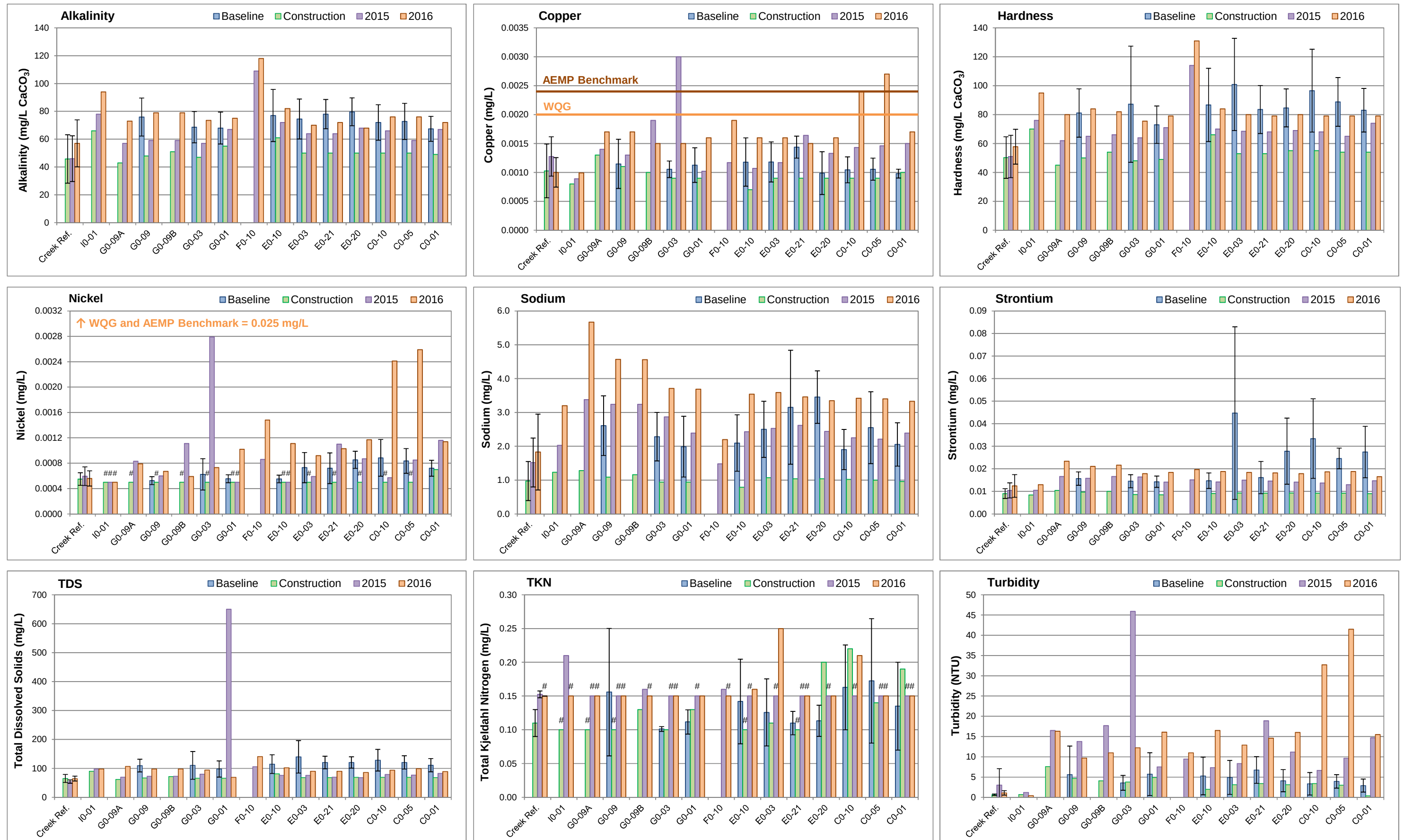
Figure C.20: Temporal comparison of water chemistry at Mary River stations for mine baseline (2005 - 2013), construction (2014) and operational (2015, 2016) periods in the fall. Values represent mean ± SD. Creek reference includes the CLT-REF and MRY-REF series stations (mean ± SD; n = 4). Pound symbol (#) indicates parameter concentration is below the laboratory method detection limit. See Table 2.2 for information regarding Water Quality Guidelines (WQG) AEMP Benchmarks are specific to Mary River.
