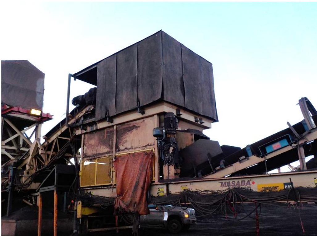
PHOTO 4 – Shrouding installed on ore crushers during 2017 to reduce dust emissions – March 2018
