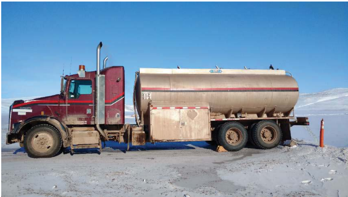
Photo 2 - Dust Suppressant water truck used to transport treated effluent
