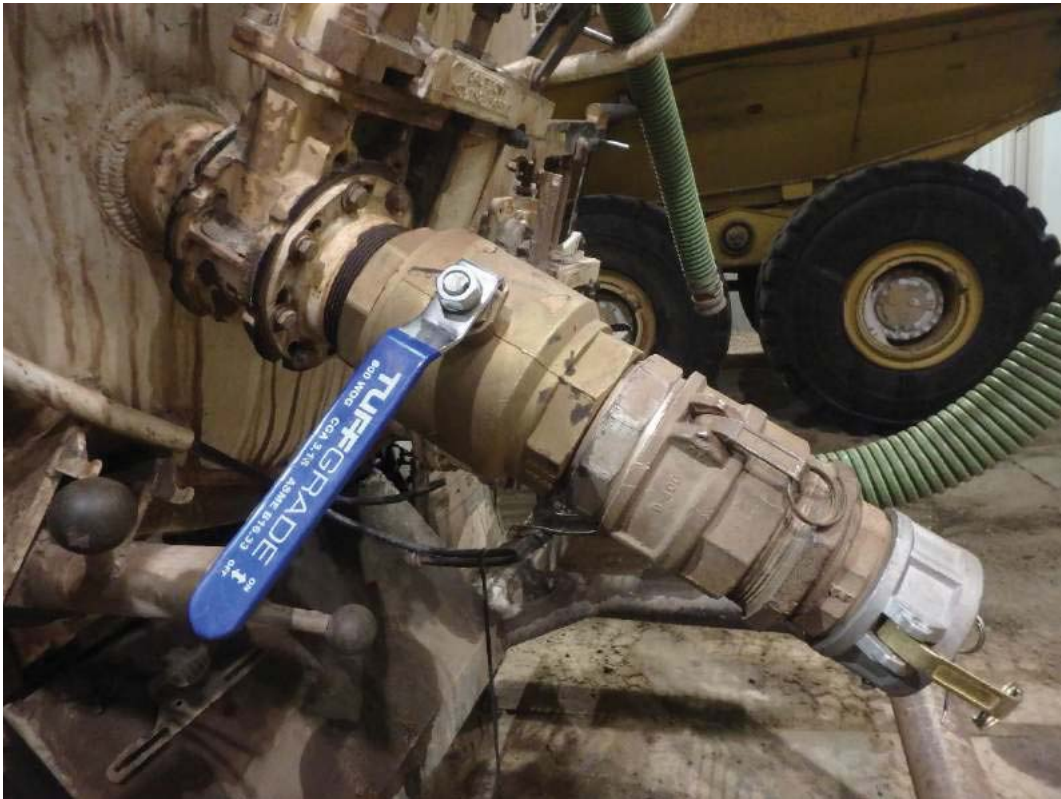
Photo 3 – New ball valve installed on the intake of the vac truck
