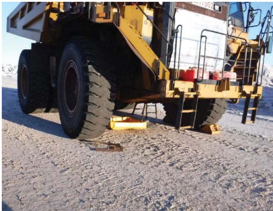
Photo 2 – Spill tray placed underneath CAT 777 while repairs were performed
