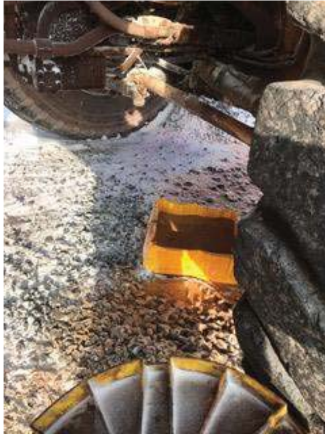
Photo 1 – Spill tray placed underneath 777 during spill
