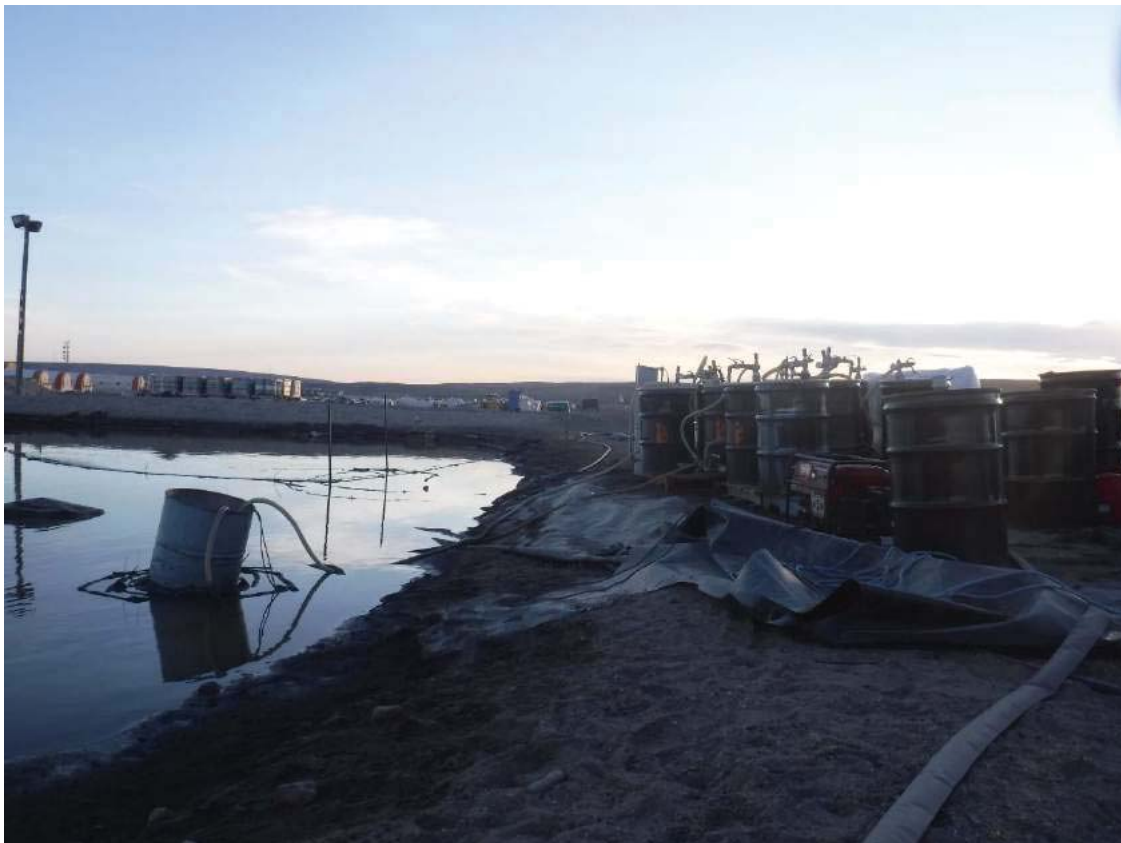
Photo 4: OWS Processing Contaminated Water in MS Old Fuel Bladder Farm (HWB 7)
