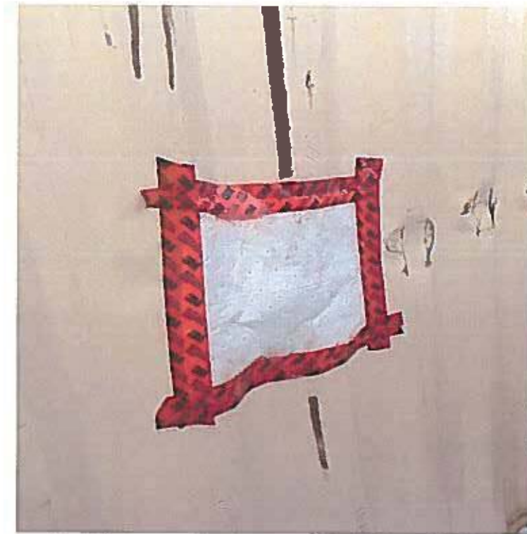
Photo 1: Sea-can puncture sealed with Absorbent Pad
