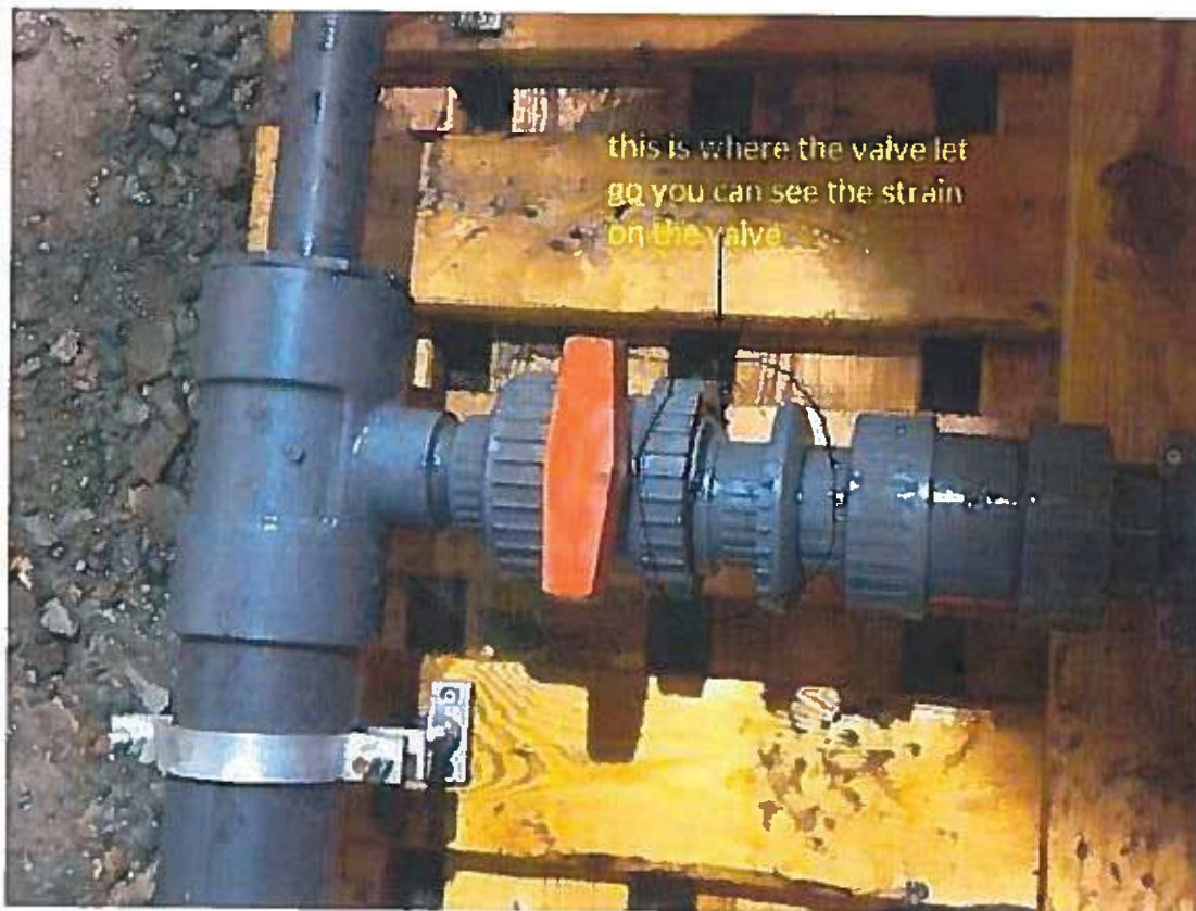
Photo 2: Broken valve from stress strain.
