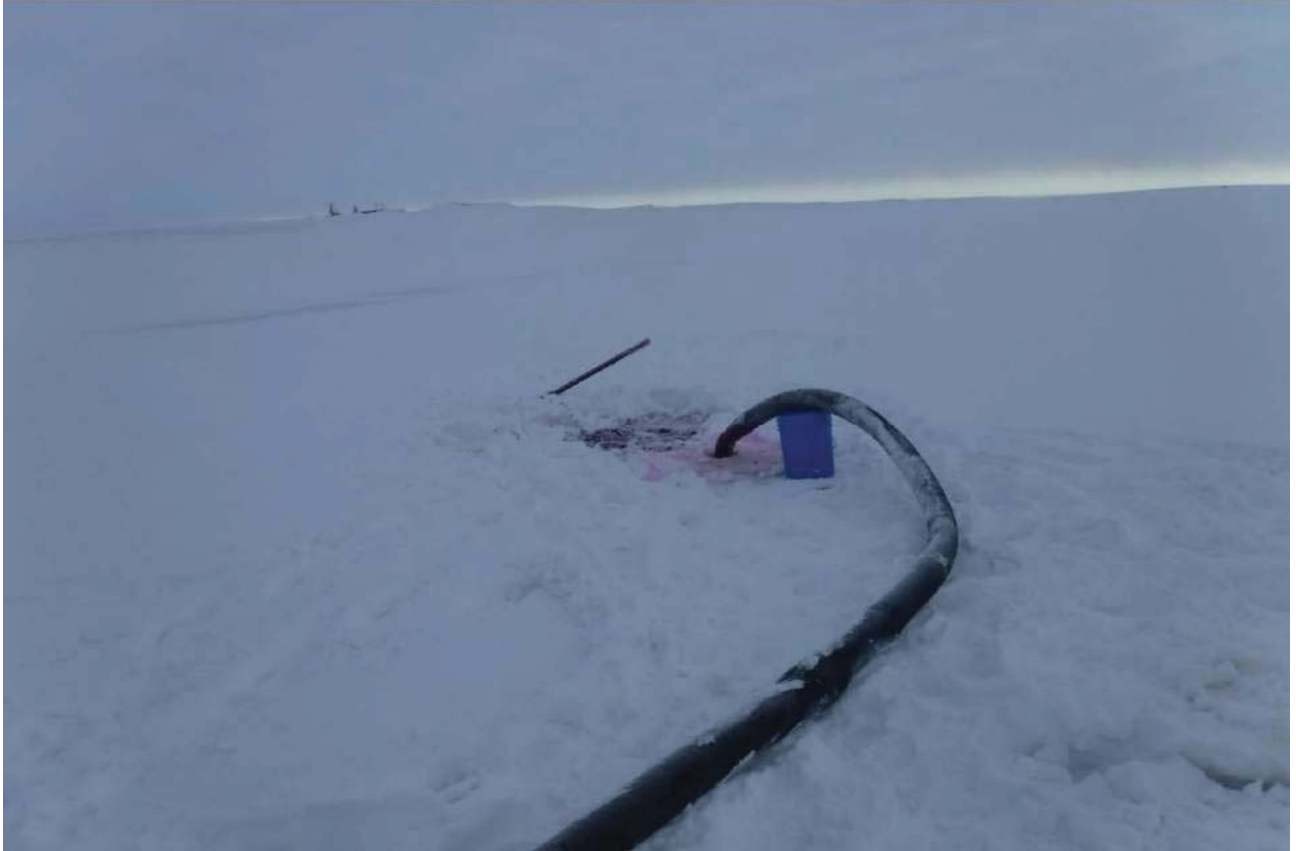
Photo 3: Recirculating Pond after Addition of Rhodamine Dye
