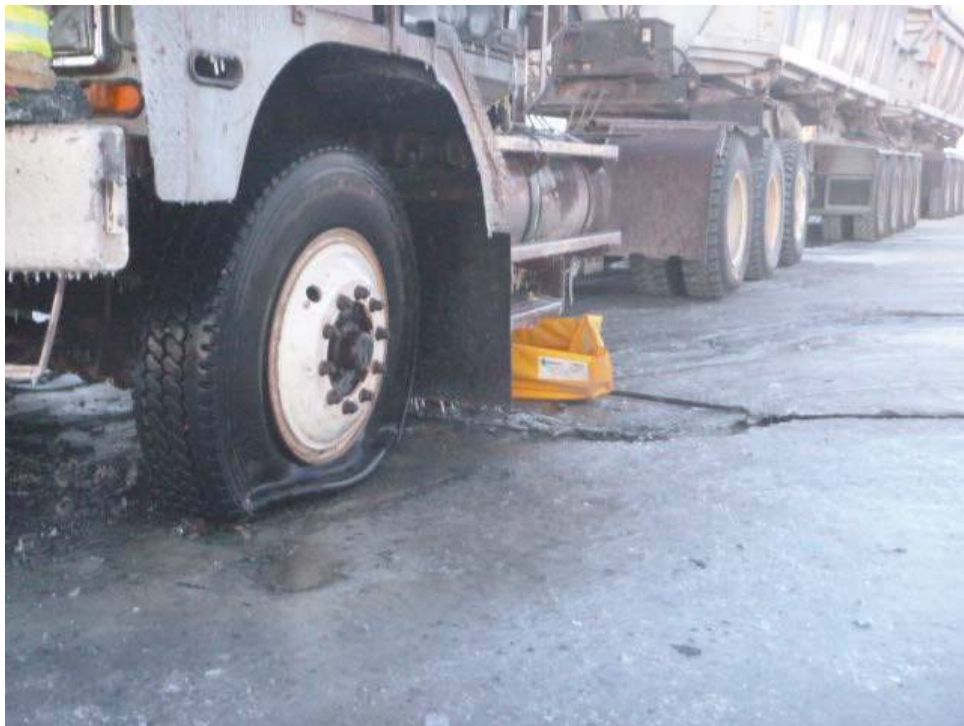
Photo 2: Ore Haul truck front cab tire- source of fire
