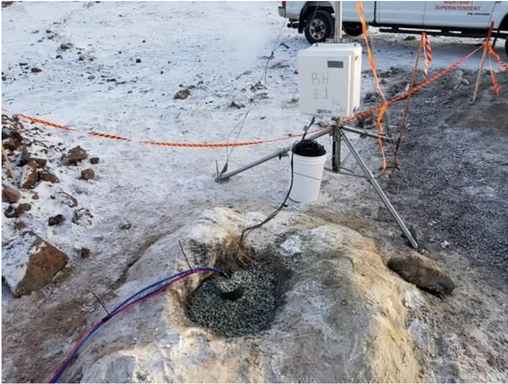
PHOTO 27 – BH 1 Borehole Final Installation O2 Sensors & Thermistors– 2019
