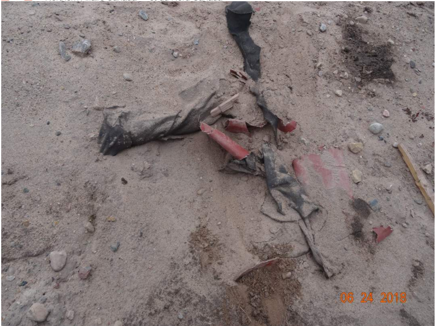
Figure 6: Hazardous waste secondary containment liner rip.
