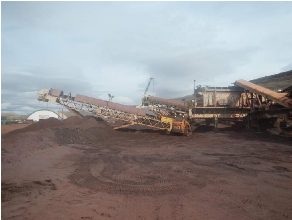
Photo 4: Ore Crusher – Transition points not enclosed to prevent dust dispersion
