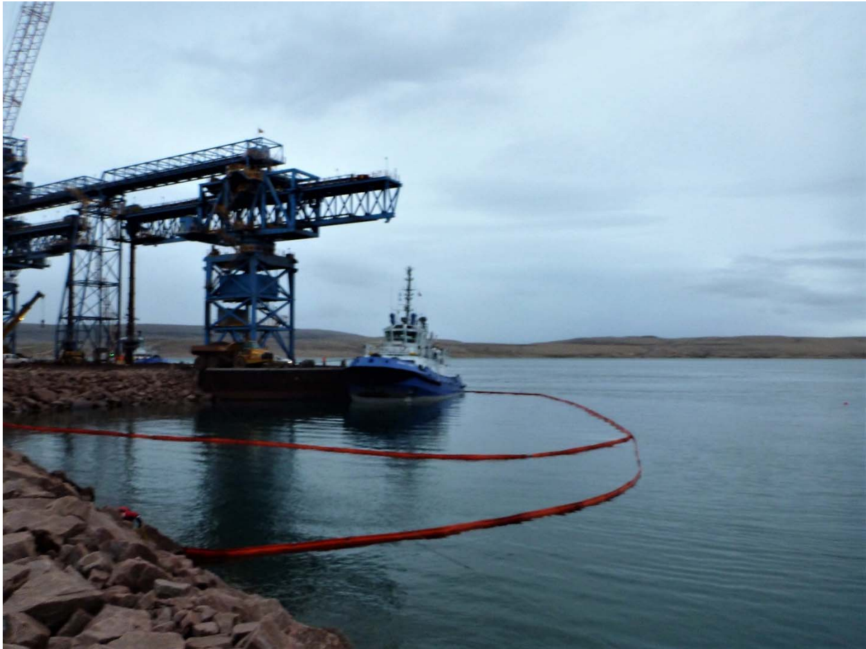
Photo 2 – July 24 th , 02:00. Vessel following relocation contained within double booms.
