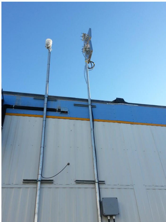
Figure 12: Milne camp WS600-UMB sensor installed on the outside wall of server room trailer (photo taken from 2014 trip)
