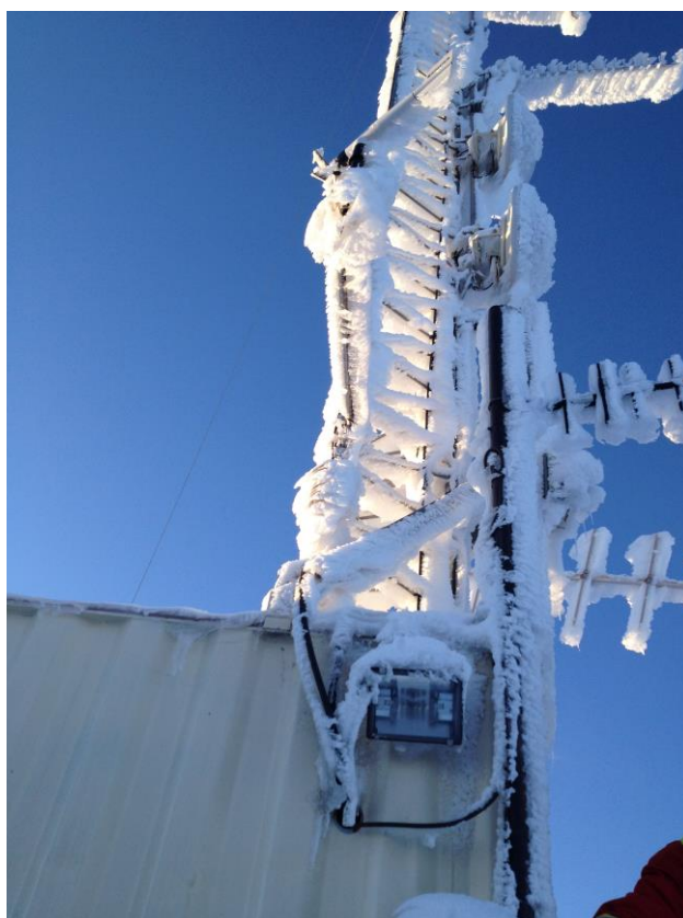
Figure 20: close up of Ice cover on Deposit No.1 sensors during 2015 trip
