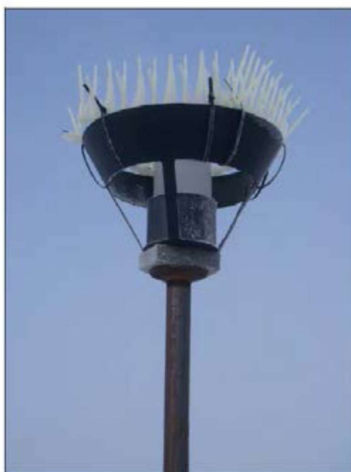
Photo 1: Dustfall collector sampling apparatus (from Rescan 2012).
