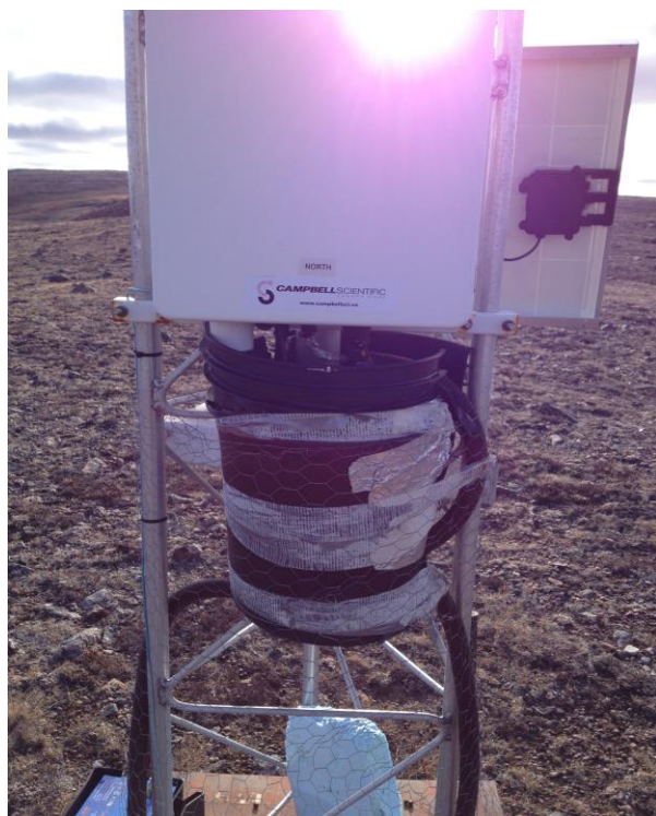
Figure 4: Supplementary chicken wire added to base of Milne station during 2015 maintenance trip
