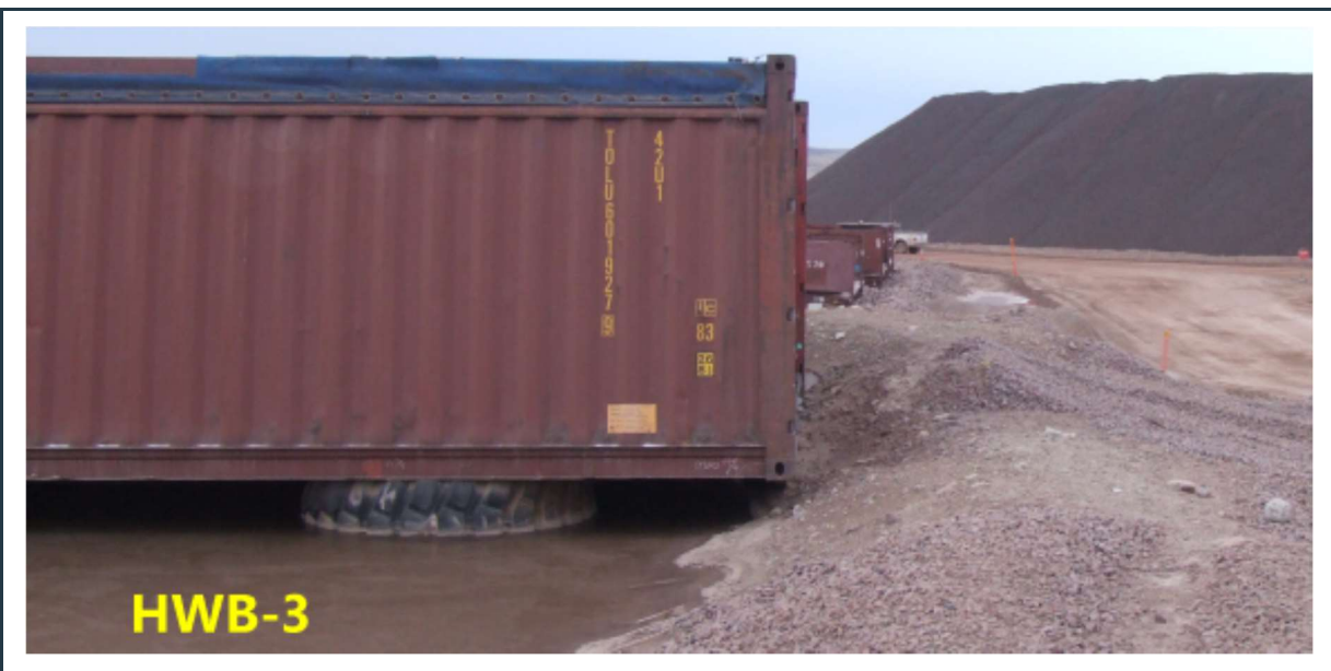
Figure 42: View of the HWB-3 cell, containing frozen water and shipping containers.
