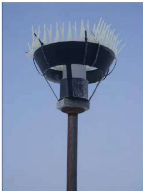
Photo 1: Dustfall collector sampling apparatus (from Rescan 2012).
