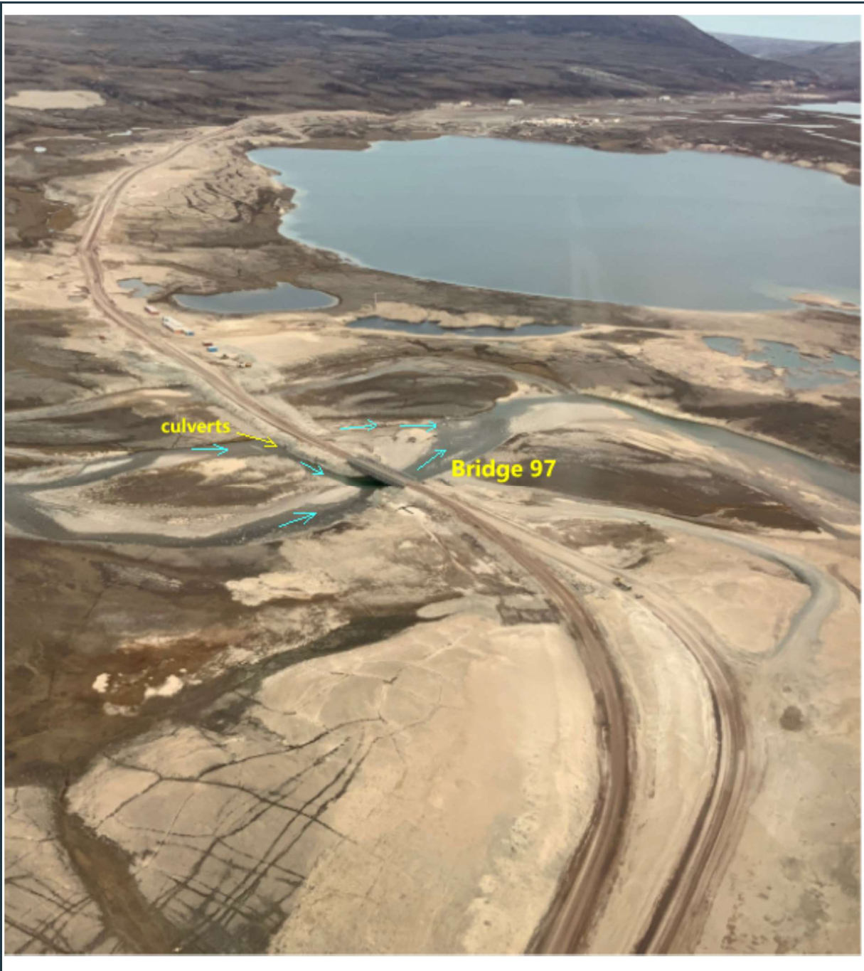
Figure 8: View of a section of the Tote Road between the Mary River Mine site and Milne Inlet Port (looking south). Bridge 97 is seen in the center, with two culverts just south of the bridge.
