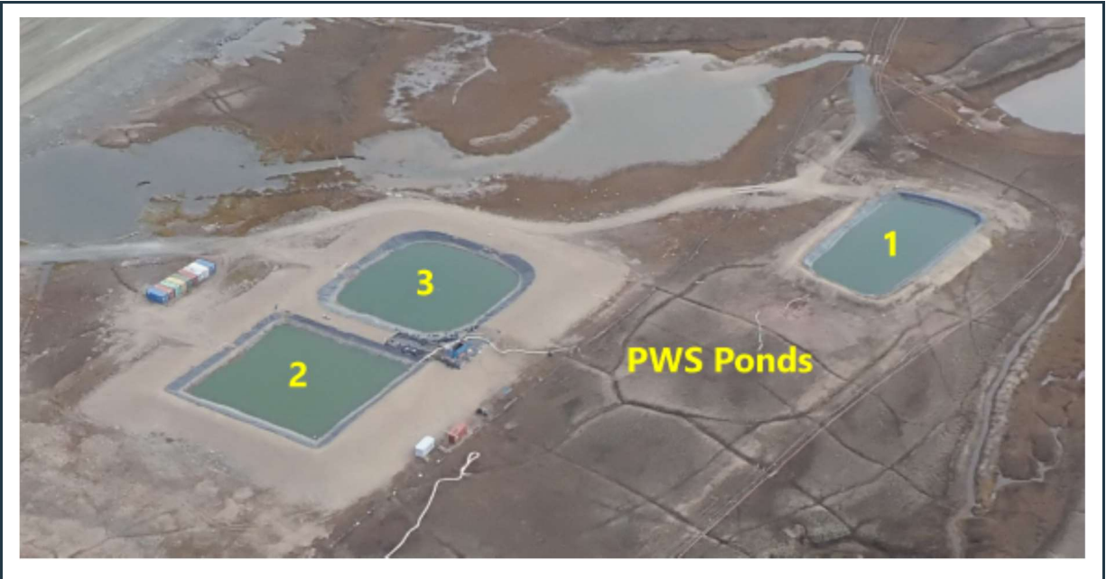
Figure 9: Aerial view of the stable berms around the three PWS ponds.
