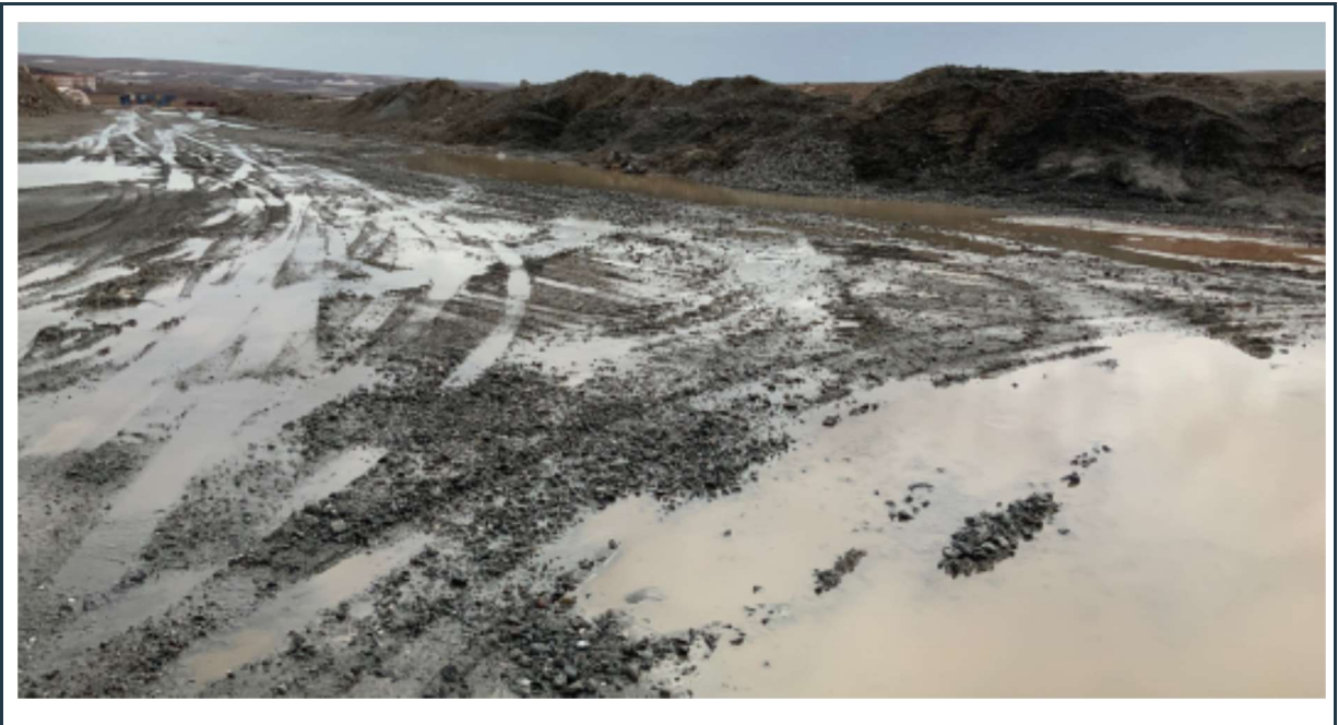
Figure 47: Poor surface water control at the main level of QMR2 quarry (enlarged from Figure 45).
