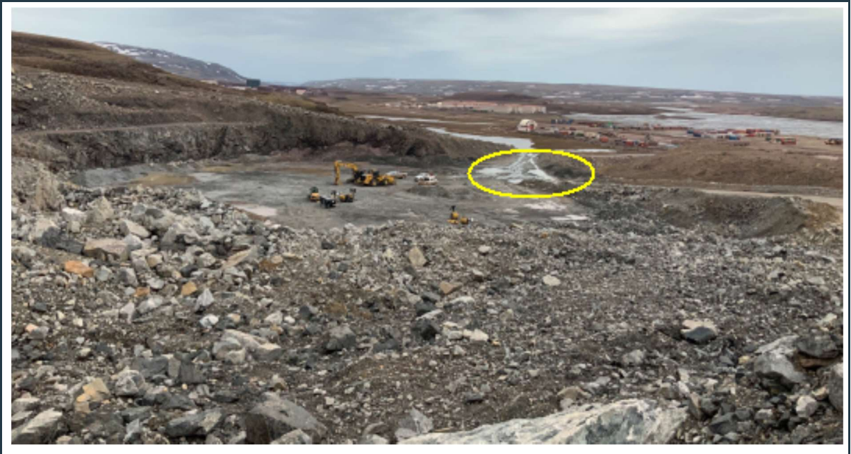
Figure 45: View of QMR2 quarry with poor surface water control area marked by the yellow circle.
