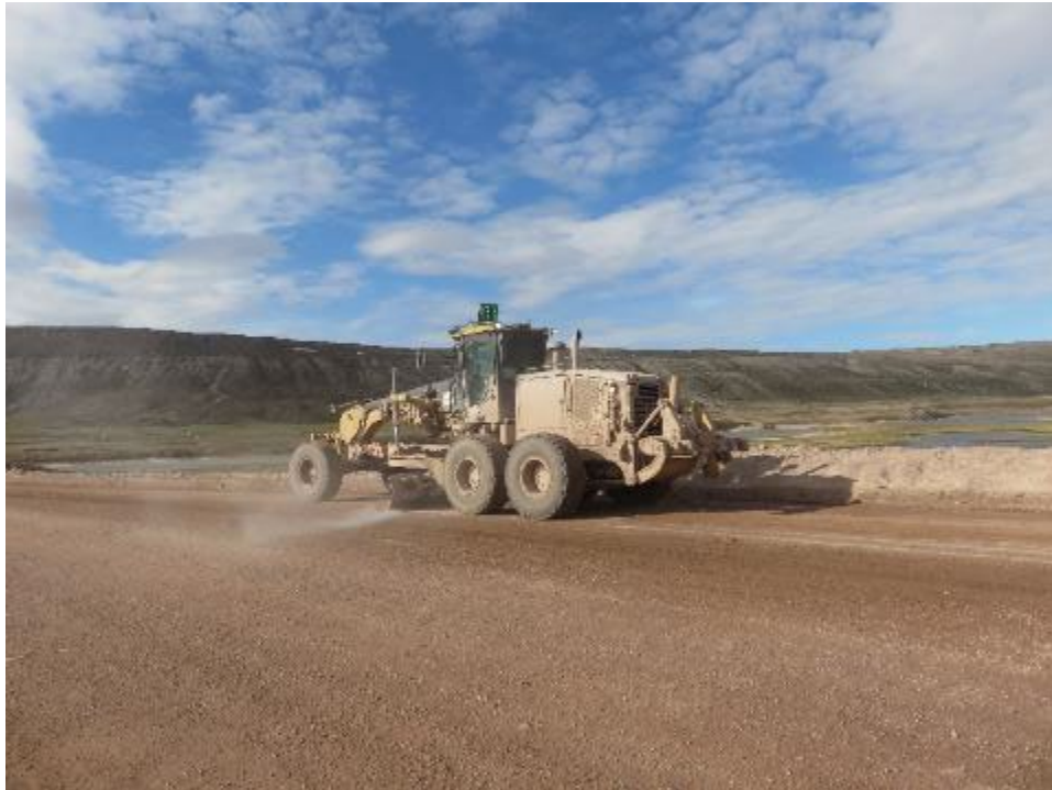
Photo 19 – Grader Maintaining Tote Road Surface – August 2021
