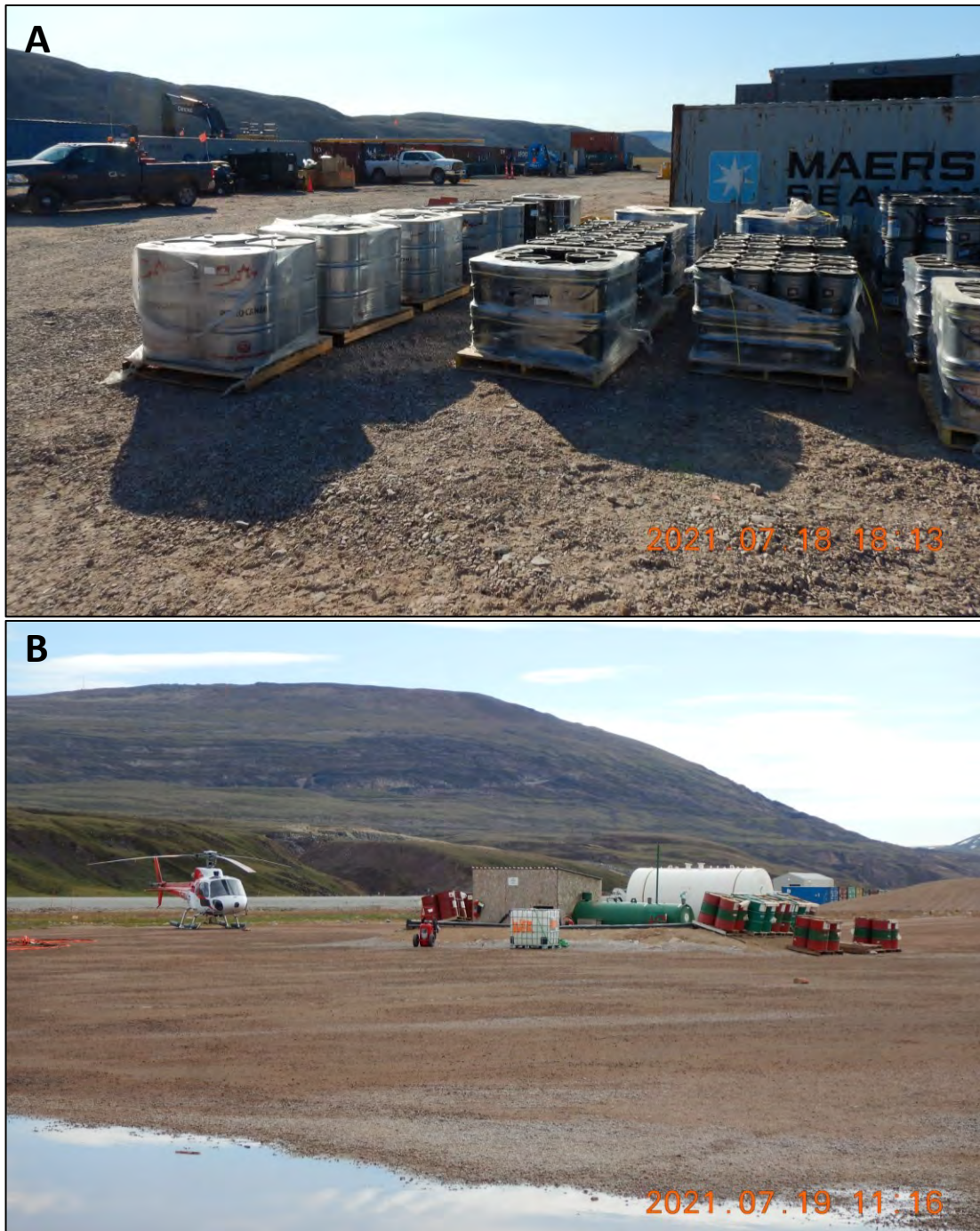
Photo 27. Fuel drums stored outside of containment at A) Qikiqtaaluk Sana laydown (KM 5) and B) Fuel drums stored outside of containment at the mine site helipad.
