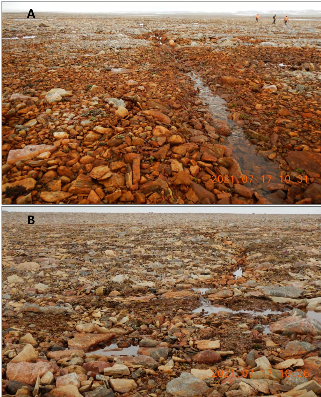
Photo 3. Formation of preferential flow path, degrading permafrost and iron staining downgradient of Waste Rock Facility Final Discharge Point approximately A) 30 m and B) 140 m down gradient.
