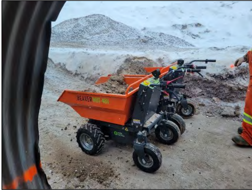
PHOTO 31. Equipment - Ducar Motorized Wheelbarrow loaded with Coarse Riprap - CV-059 (April 04, 2024).
