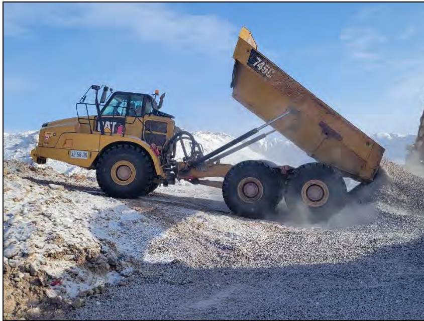
PHOTO 31. Equipment - CAT 745C articulated dump truck - km 80 Laydown (April 23, 2024).
