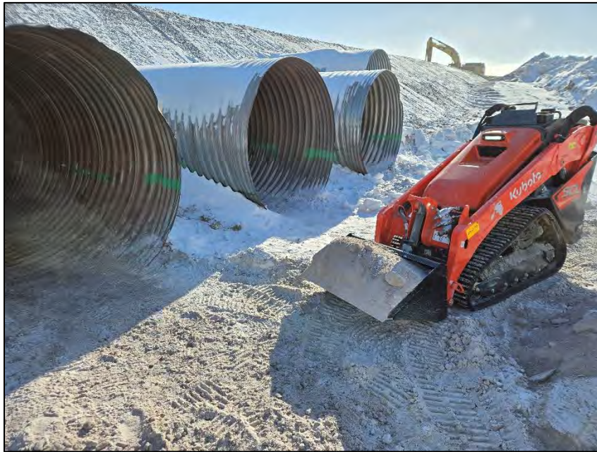
PHOTO 33. Equipment - Kubota SCL 100 Stand On Compact Loader - km 80 laydown (May 01, 2024).
