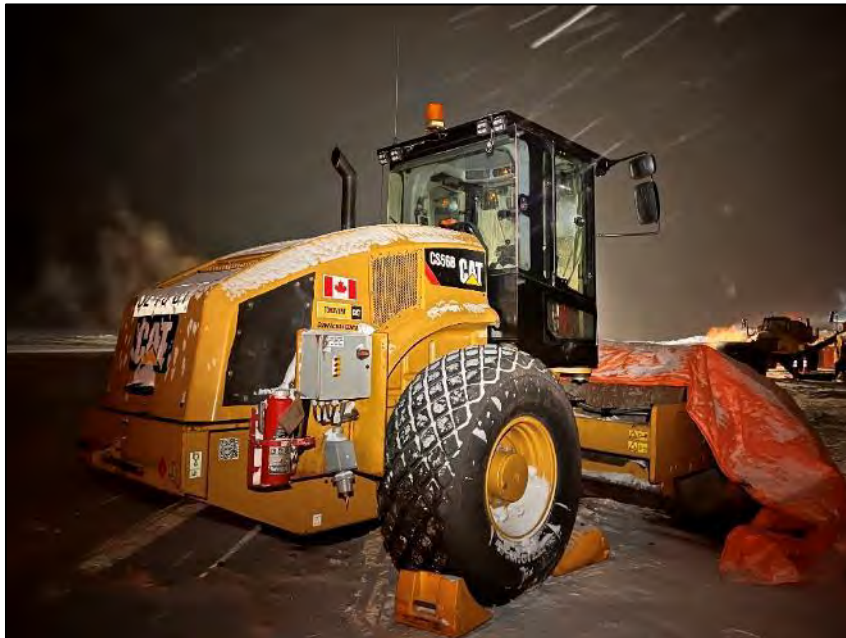
PHOTO 32. Equipment - CAT CS56B Smooth Drum Compactor (March 02, 2024).
