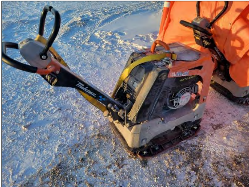
PHOTO 28. Equipment - Mikasa MVH408 1000 lb Plate Compactor - km 60 Laydown (March 05, 2024).
