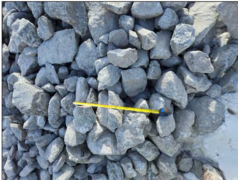
PHOTO 28. Material Stockpile - Fine Rip Rap - km 80 Laydown (May 01, 2024).
