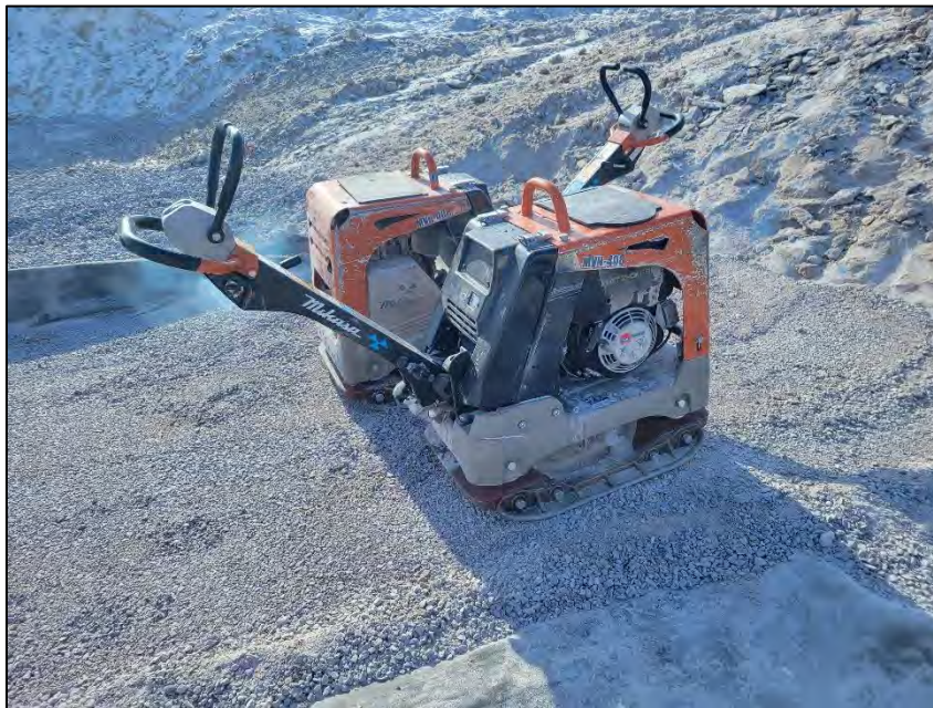
PHOTO 32. Equipment - Mikasa MVH408 1000 lbs Plate Compactor - km 80 Laydown (April 20, 2024).
