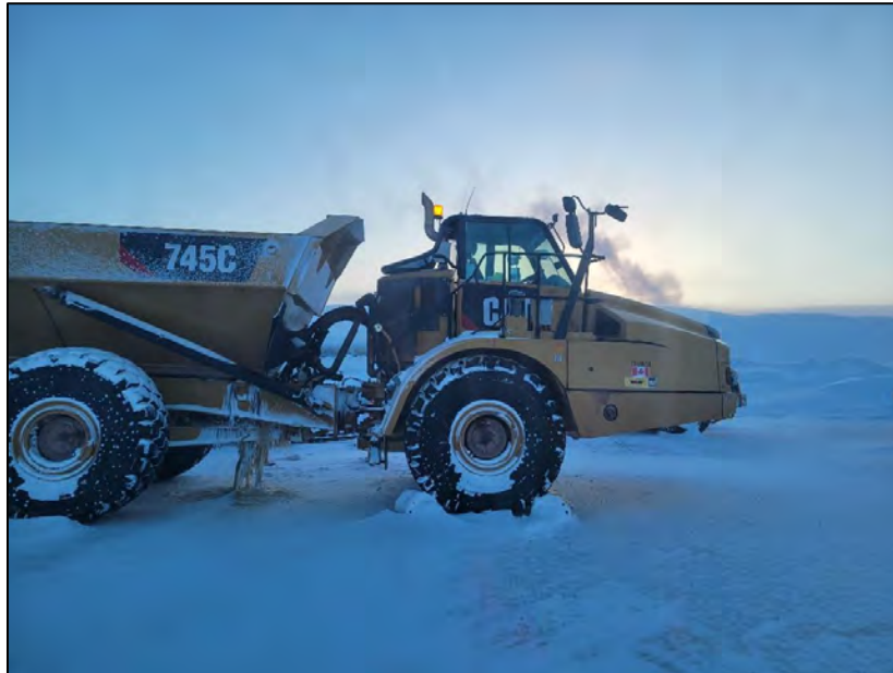
PHOTO 31. Equipment - CAT 745C articulated dump truck - km 60 laydown (February 8, 2024).
