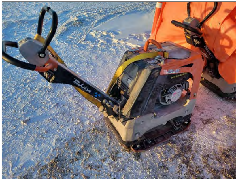
PHOTO 32. Equipment - Mikasa MVH408 1000 lb plate compactor - km 60 laydown (March 5, 2024).
