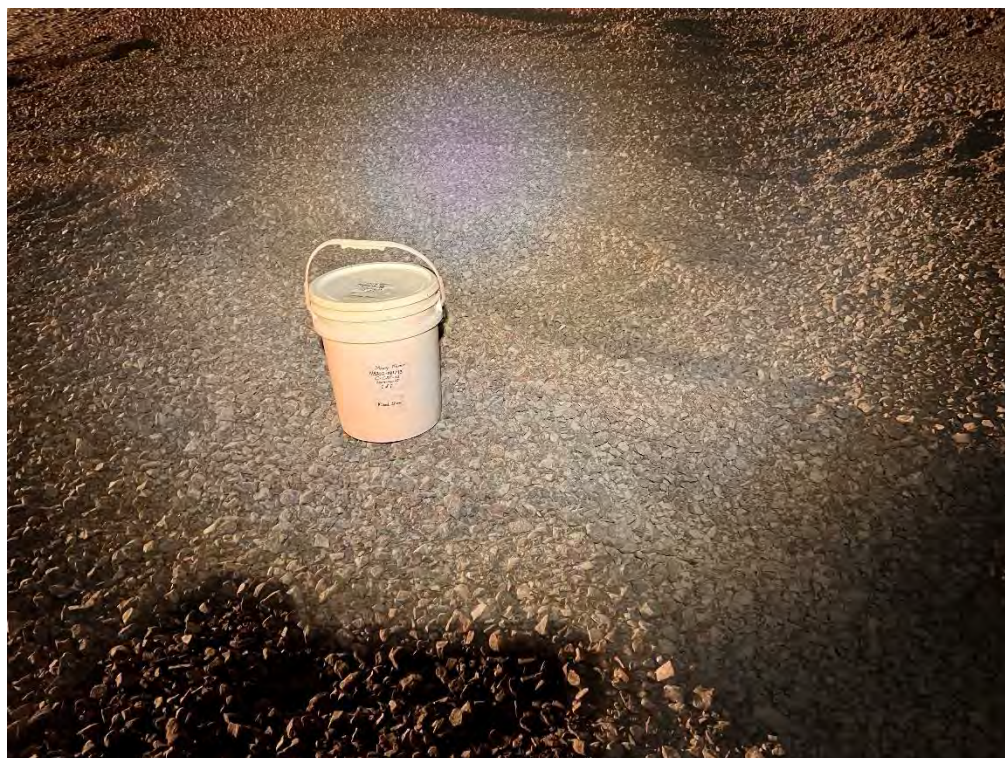
Photo 16: Control sample collected from 32 mm minus stockpile at km 60 (February 23, 2024)
