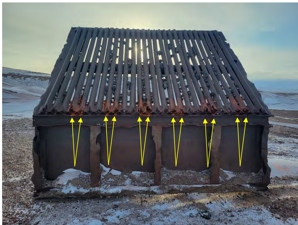
Photo 6: Grizzly screen with bars to be removed painted orange
