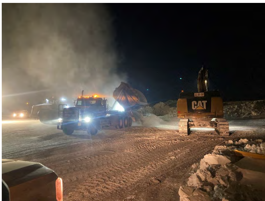
Photo 10 Ore hauling truck (OHT) transporting 32 mm minus material from Milne Port to the 60 km laydown stockpile. Photo taken March 16, 2024.
