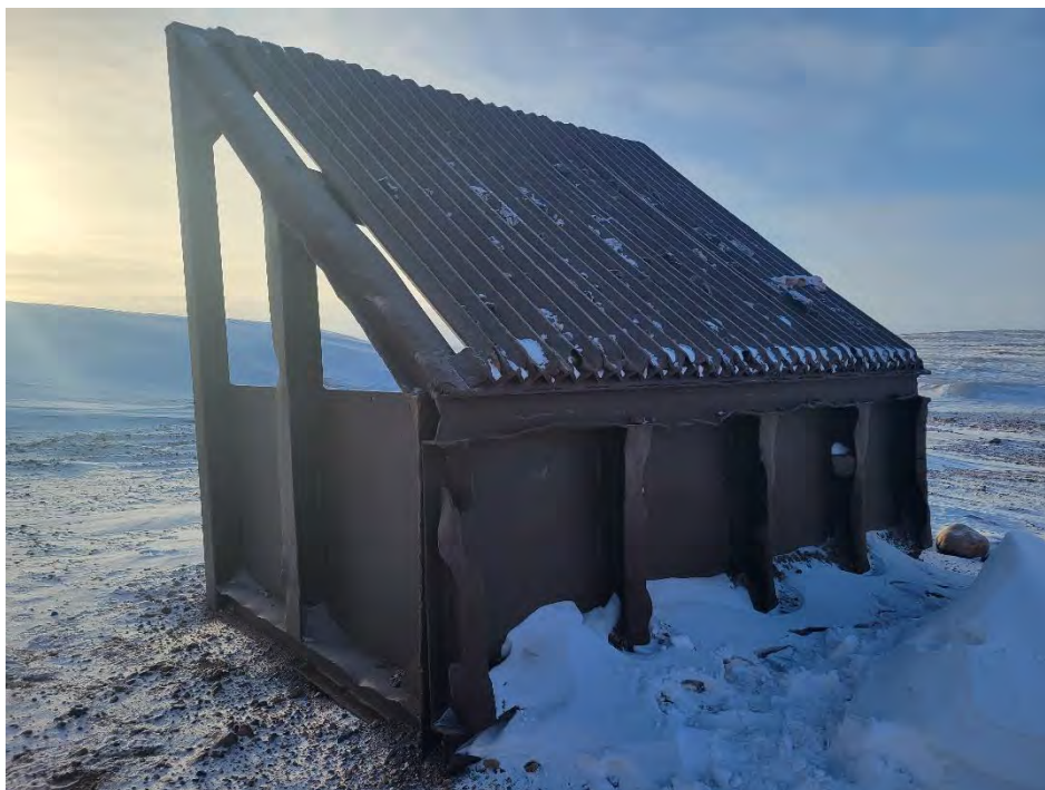
Photo 5: Grizzly Stream to be modified for sorting of the Coarse Riprap
