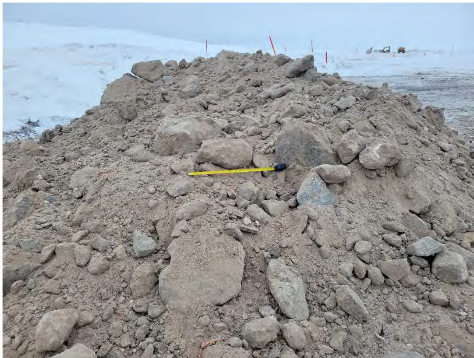
Photo 14 Zoomed out sizing of common borrow material used outside of 32 mm minus trapezoid at BG-04. Photo taken April 8, 2024.
