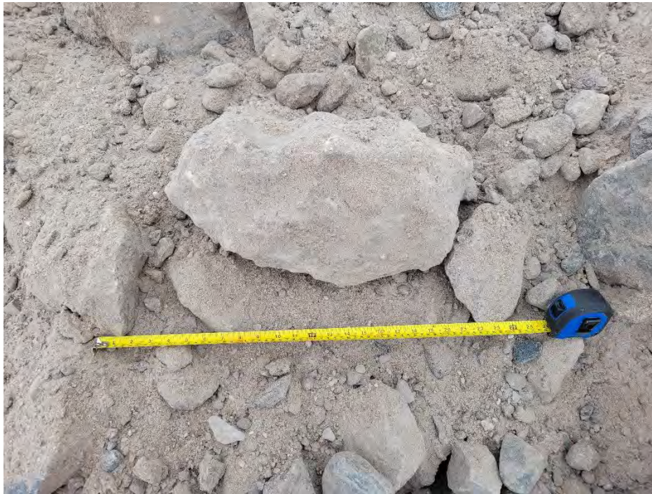
Photo 13 Zoomed in sizing of common borrow material used outside of 32 mm minus trapezoid at BG-04. Photo taken April 8, 2024.
