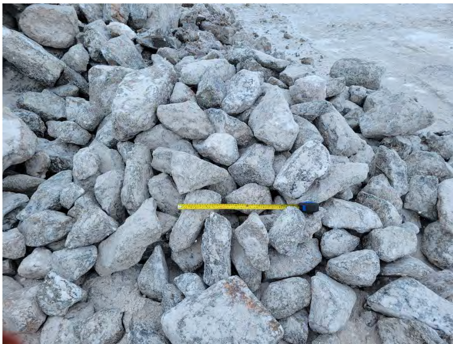
Photo 30 Zoomed out size of coarse riprap used at CV-001. Photo taken April 5, 2024.
