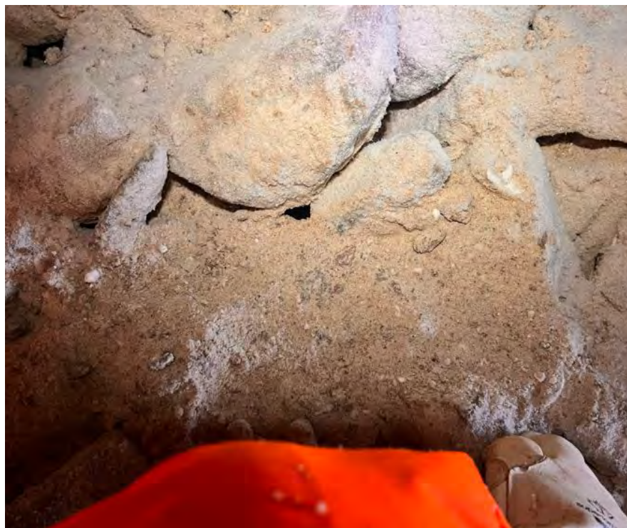
Photo 5 Snow mixed in with the Culvert Infill Material at BG-04 culvert
