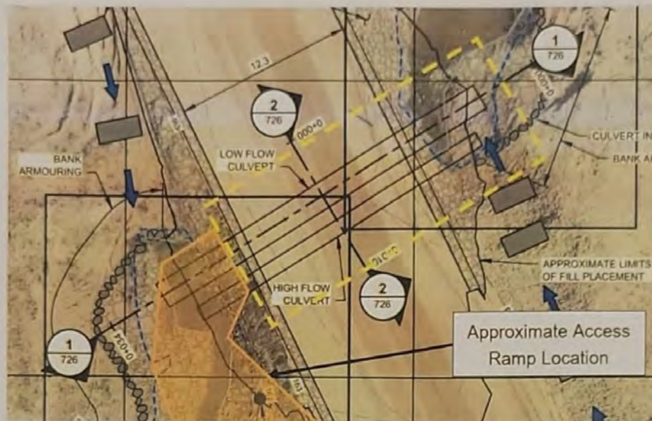
Figure 1: Approximate Foundation Acceptance Area, Plan View (Yellow dotted line).
