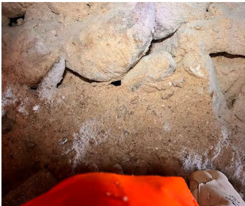
Photo 5 Snow mixed in with the Culvert Infill Material at BG-04.
