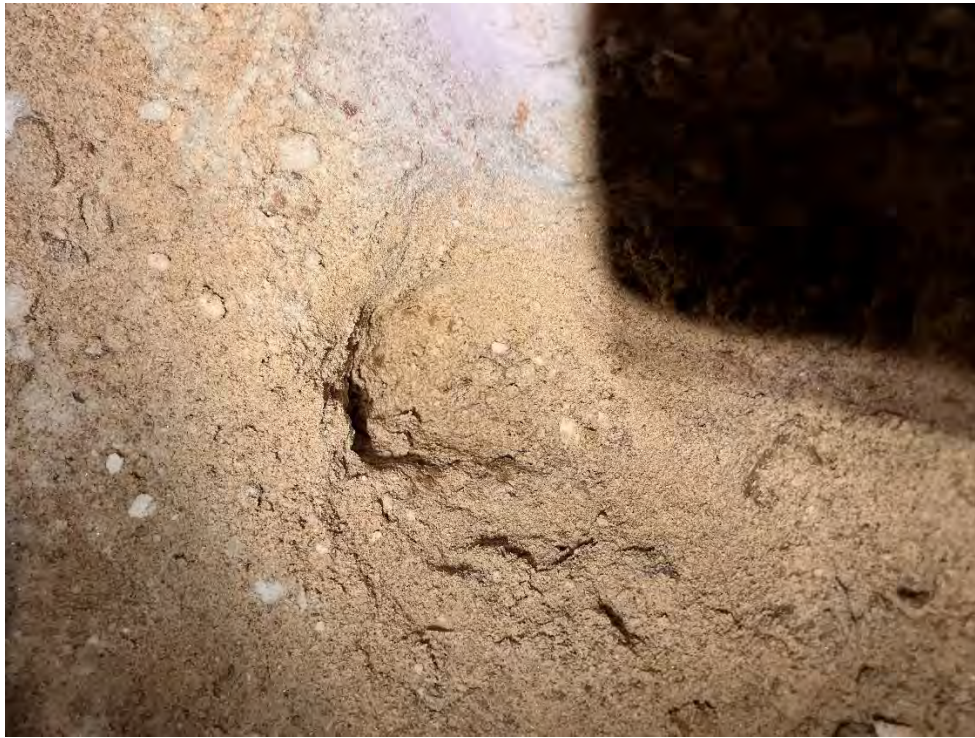
Photo 3 Hole made to inspect the snow mixed in with Culvert Infill Material at BG-04
