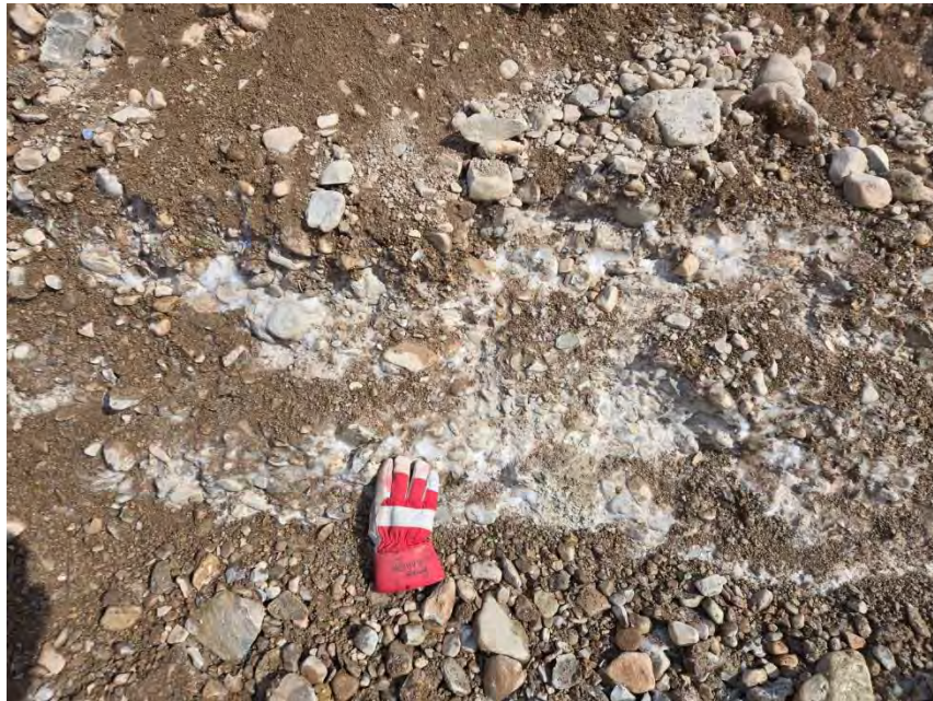
Photo 4 Ice-rich soils encountered in the foundation area. Photo taken May 5, 2024, looking east.
