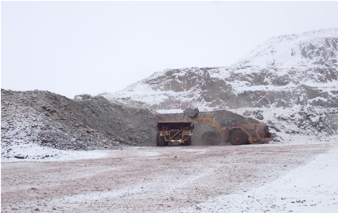
Photo 6. Loading a 570 Mine Haul Truck in Nuluujaak Pit - April 2024
