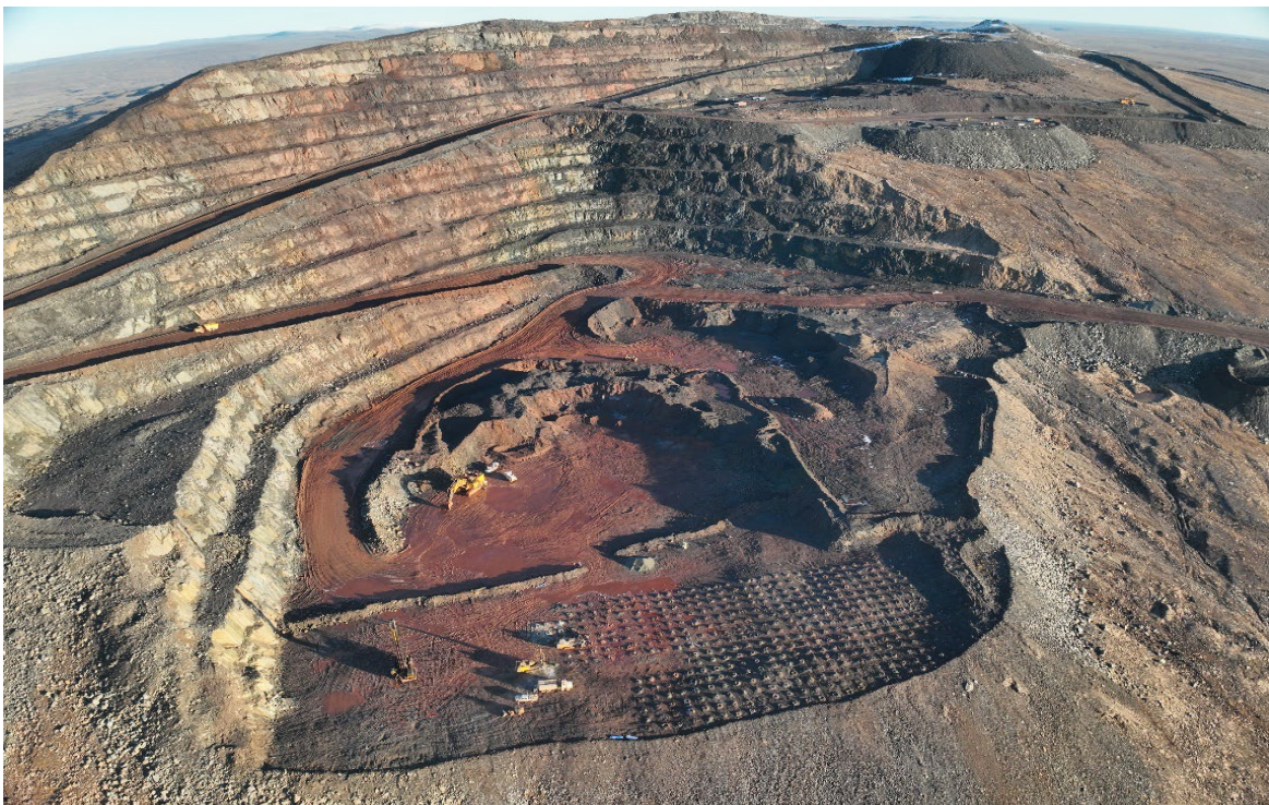
Photo 8. Drilling Blast Pattern in Nuluujaak Pit - September
