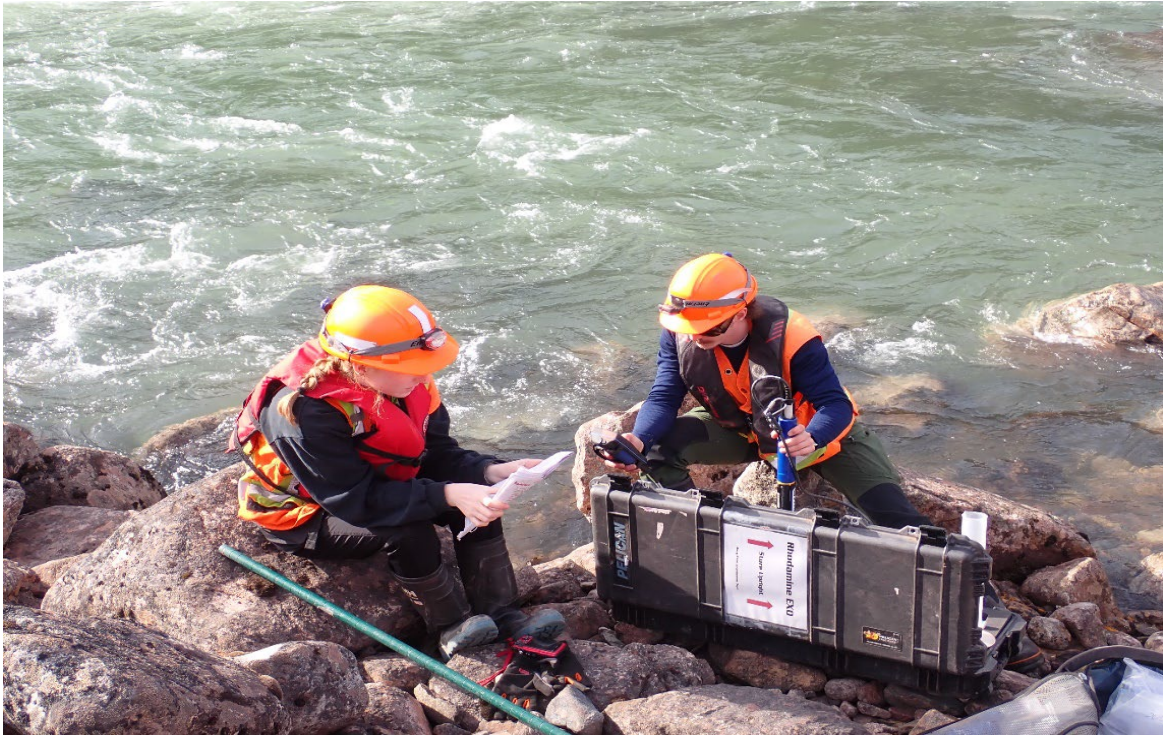
Photo 61. Hydrology Rhodamine Water Flow Survey - July
