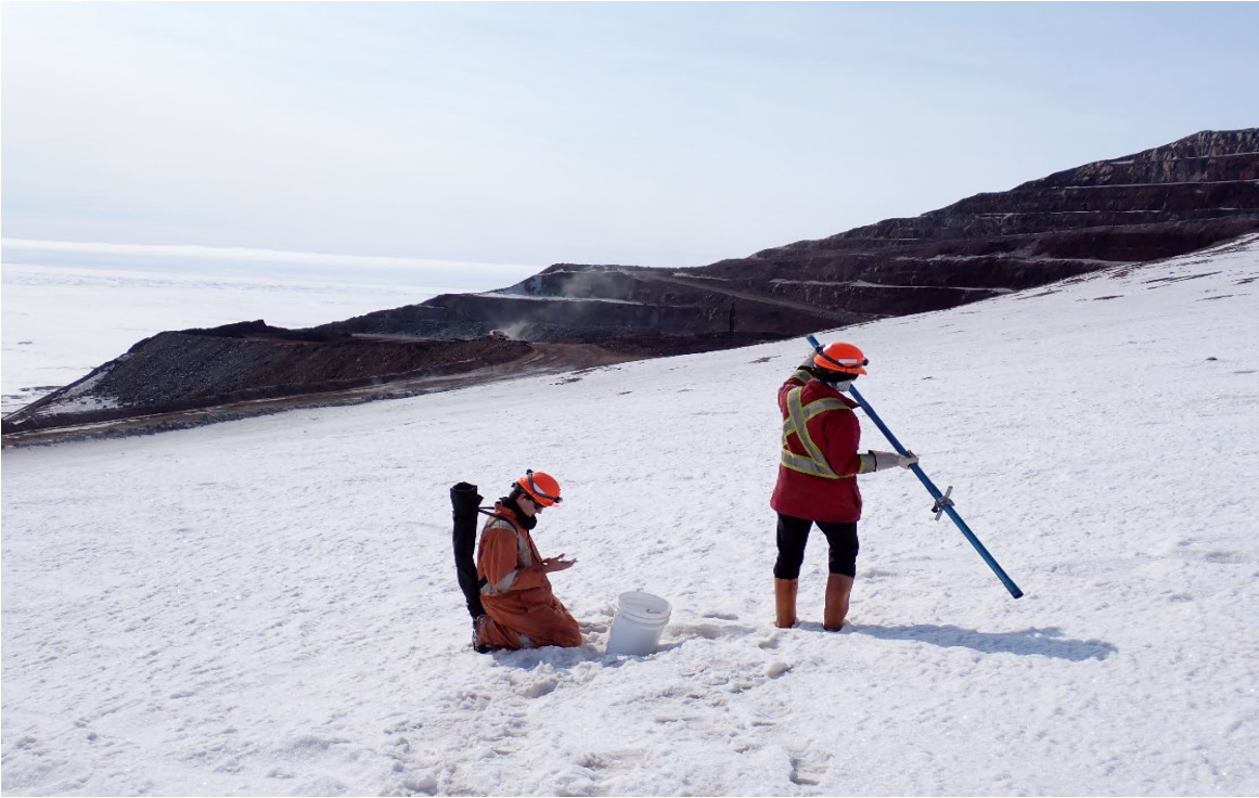
Photo 80. Snow Core Sample Collection East of Deposit 1 - May
