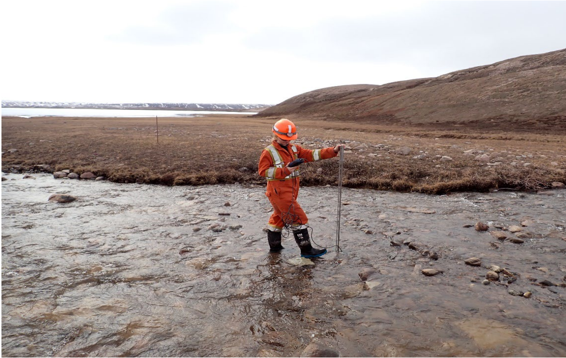
Photo 63. SNP Measuring Stream Depth and Velocity - May
