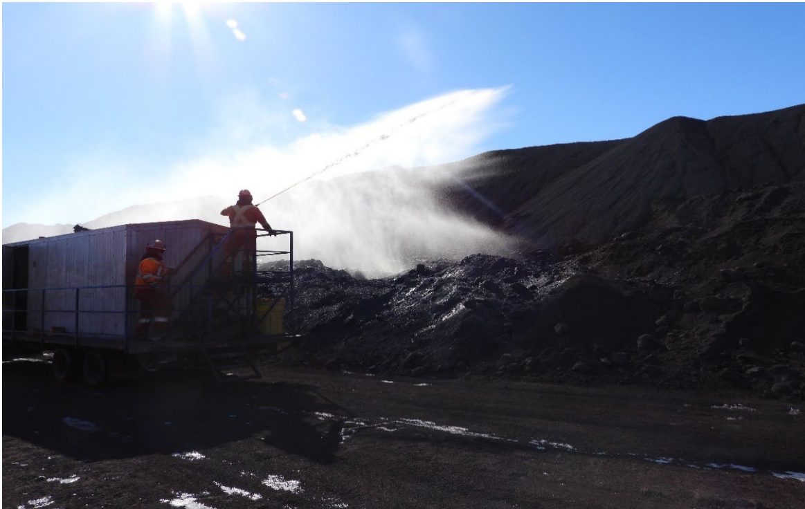
Photo 33. Dust Suppression Being Applied to the Ore Pad stockpile – May
