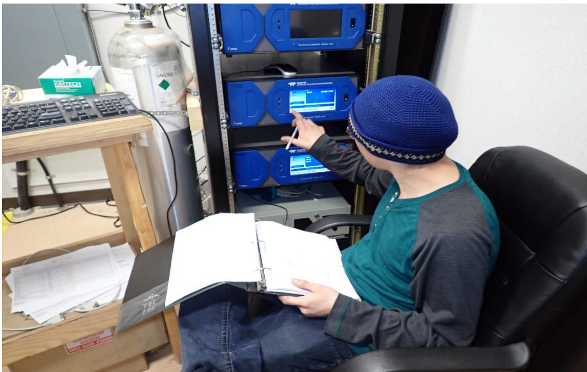
Photo 31. Beta Attenuation Monitor (BAM 1020) Unit Inside Port Site Complex (PSC) – December
