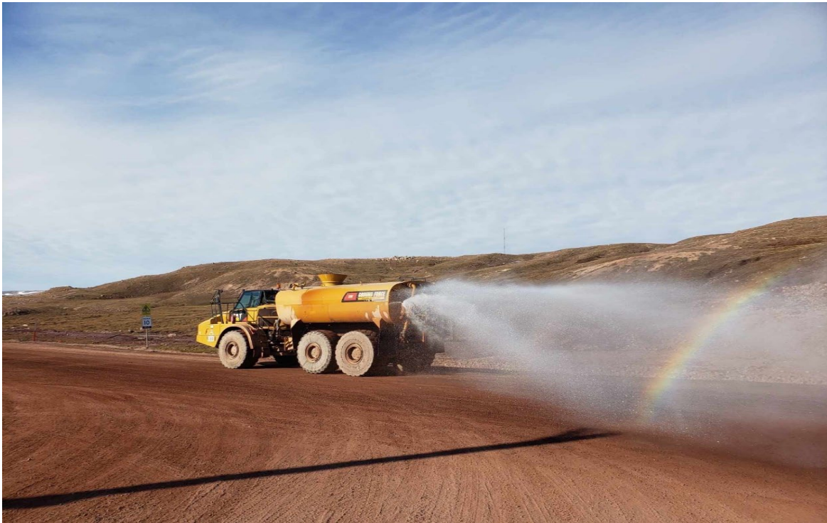
Photo 34. 740 Water Truck Applying Water as Dust Supressant on the Tote Road – June
