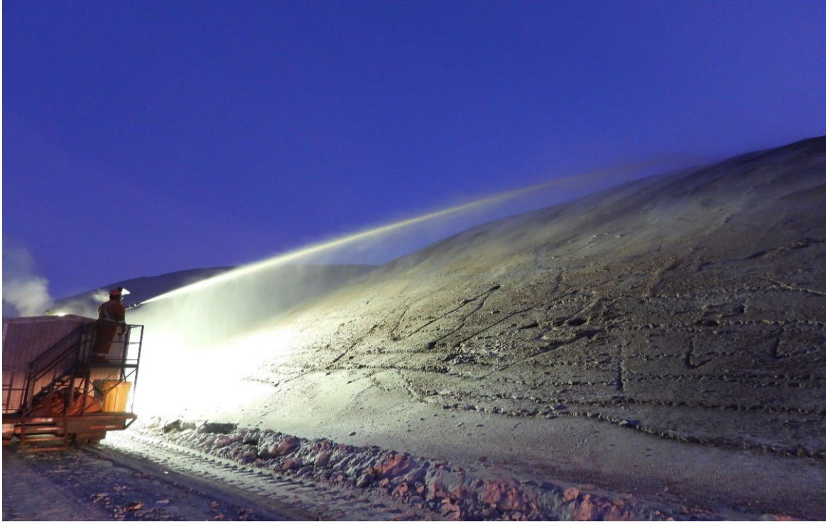
Photo 32. Dust Suppression Being Applied to the Ore Pad Stockpile – January
