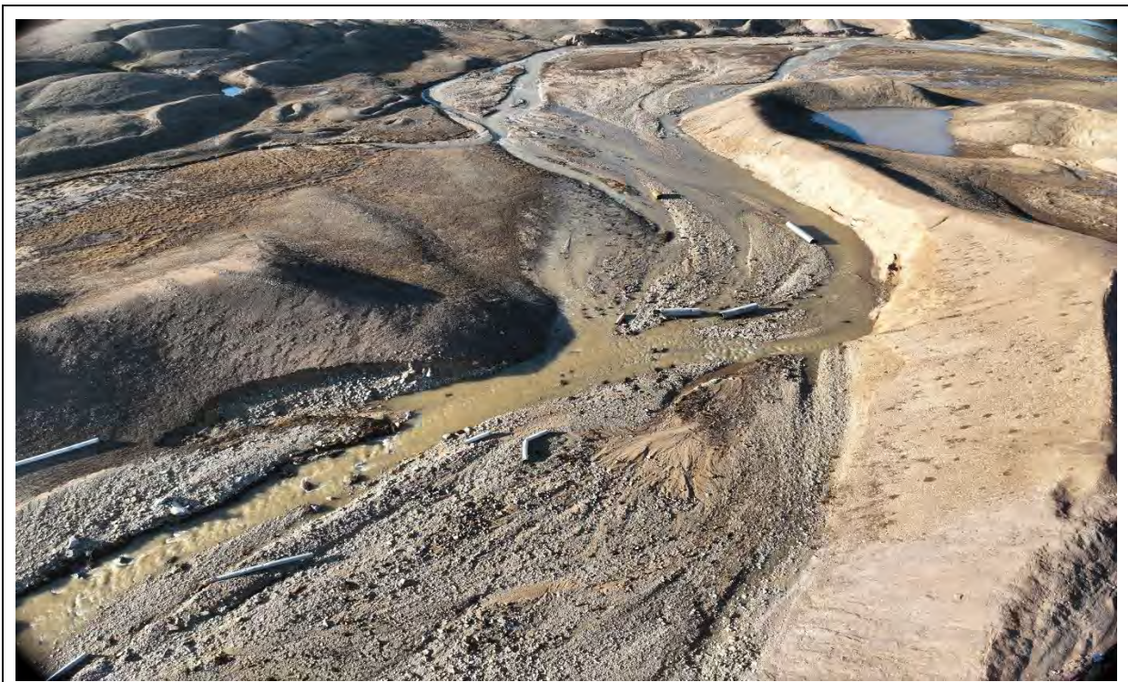
Photo 2. KM 63.5, Culverts deposited downstream from Tote Road crossing during September rain event, 2024-09-22
