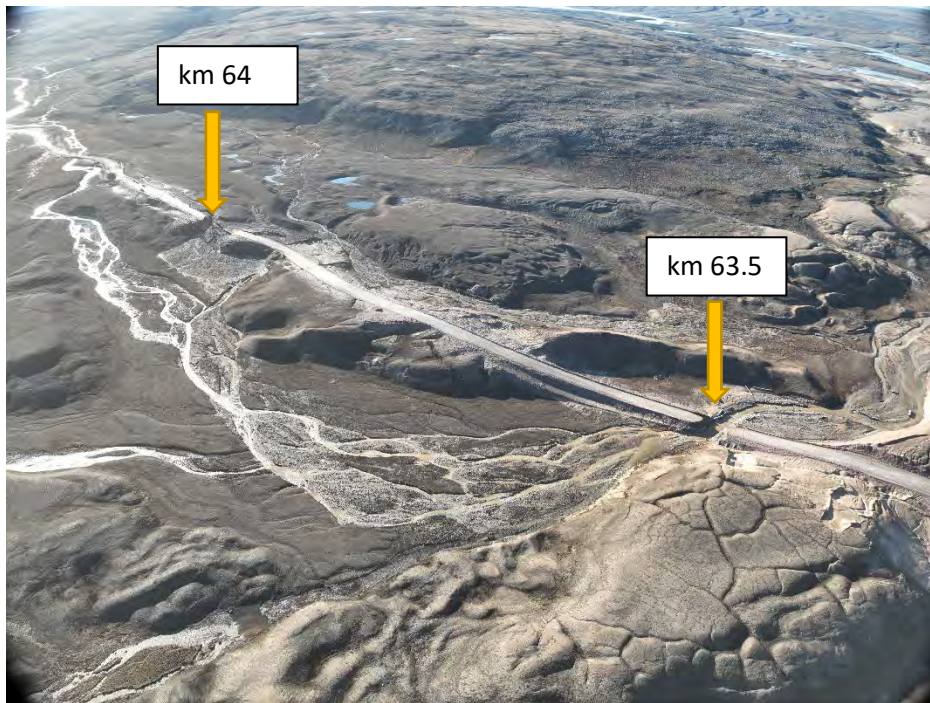
Photo 4: km 64/63.5 Aerial Photo Showing Damage to Roadway following Rainfall Event (September 23)
