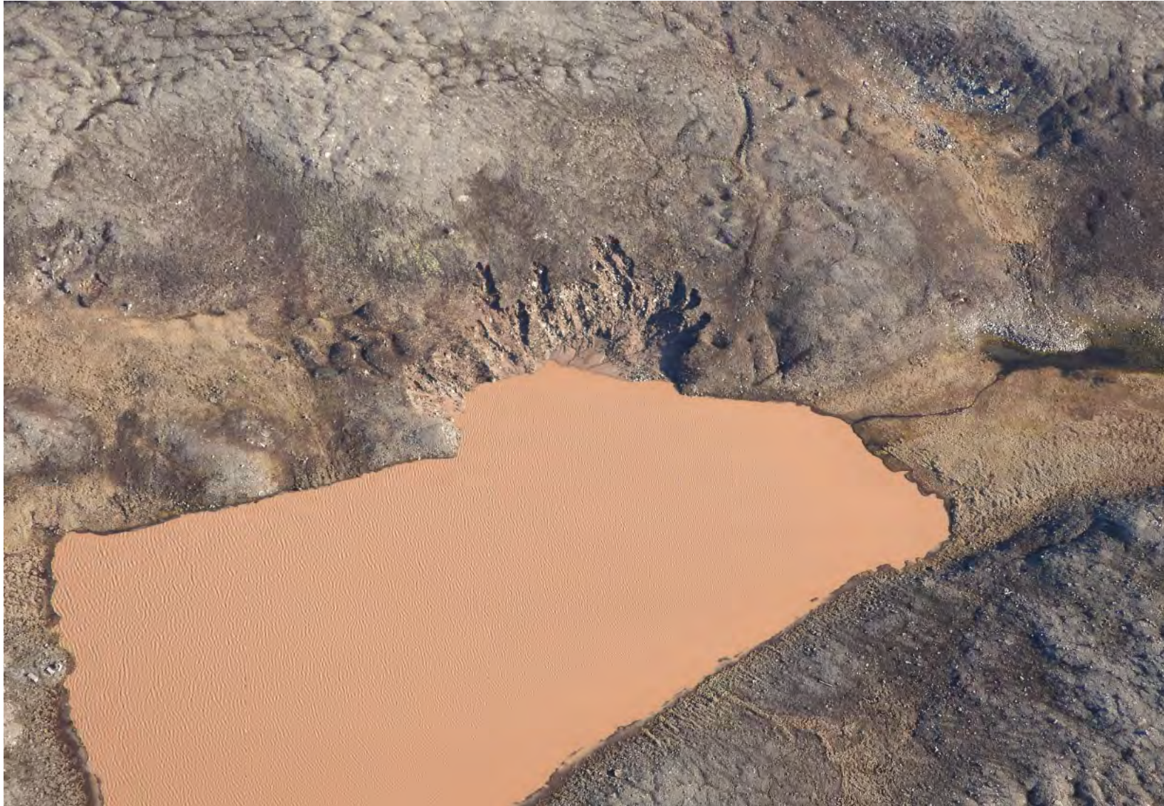
Photo 3: Slope failure into unnamed lake, resulting in apparent iron-rich TSS loadings to lake 9 km NW of Project, 2024-09-24.
