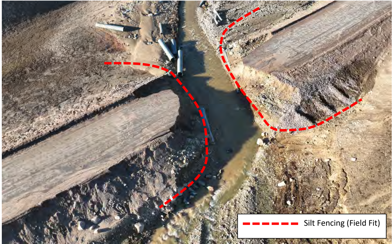
Figure 2: ESC plan for km 63.5 work adjacent to water
