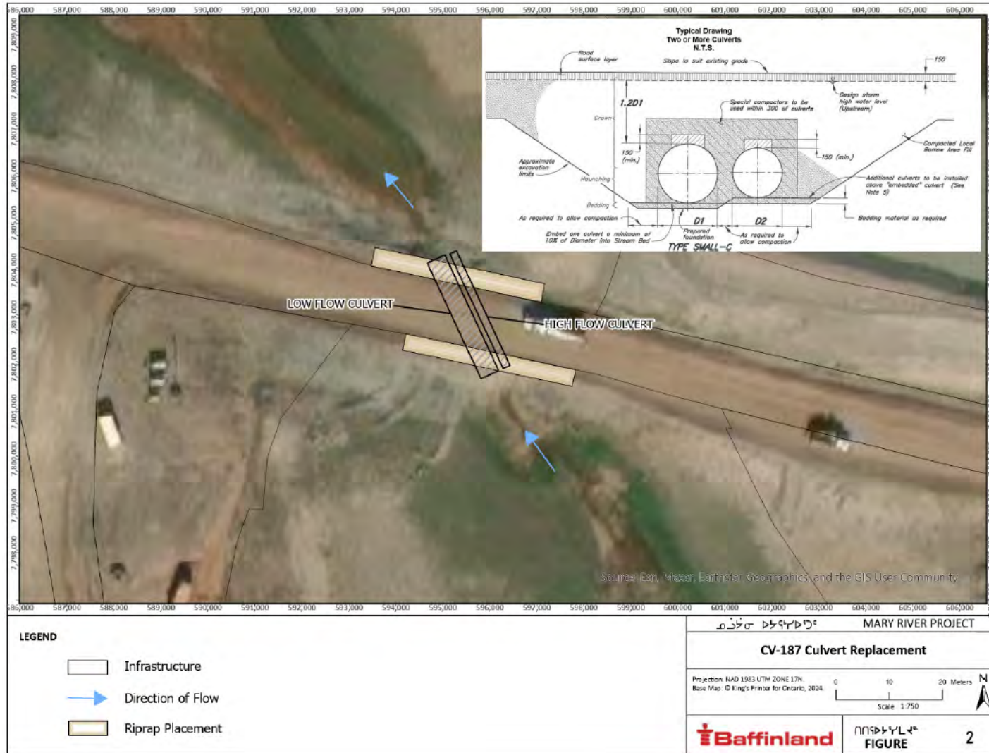
Figure 2. IFC Drawing for CV-187 Culvert Replacement
